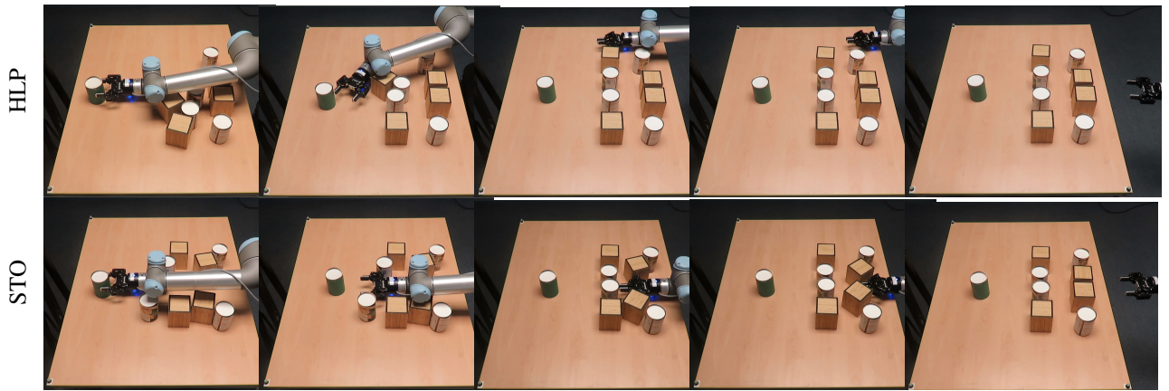
Fig. 5: Human-like Manipulation (HLP) plan (top), and Baseline (STO) plan (bottom). HLP algorithm can reason over the task space and navigate through the free space around the obstacles similar to what people may do. On the other hand, STO is biased towards its straight-line initialization and hence had to push objects around which made it 1.5 times slower than HLP.
