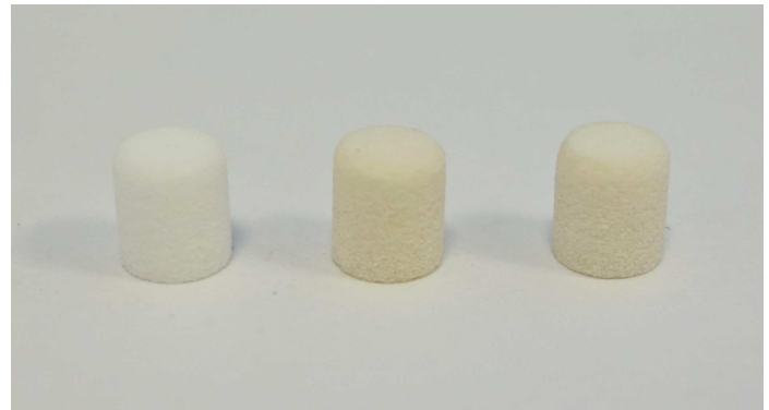
Figure 2: Photo of the specimens printed for micro-CT scanning, showing (left to right) virgin PA2200, 1% B65003 and 1% B45003.
