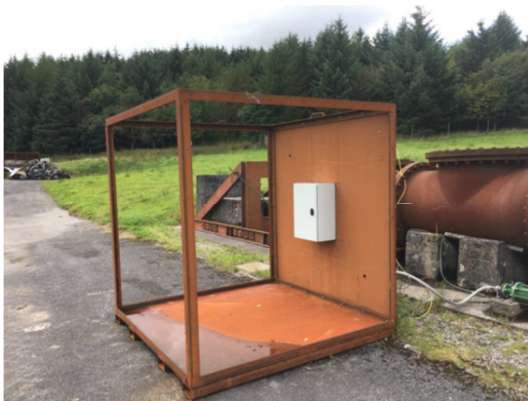
Fig. 1. Test rig in-situ with electrical box with door on in place ready for testing.
