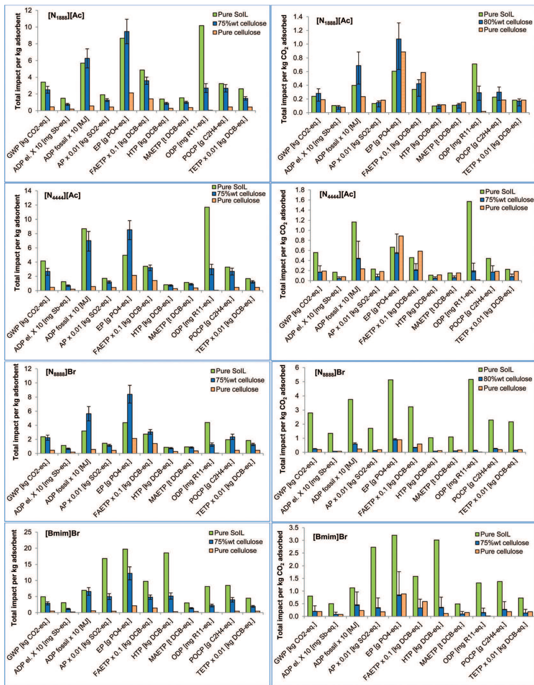
Fig. 5 Environmental impacts of pure and cellulose-supported SoILs as a function of cellulose loading: per kg of adsorbent (left) and per kg CO 2 adsorbed (right). (For impacts nomenclature, see section 3.1. The error bars represent the 70% (upper limit) and 80% cellulose loading (lower limit), except for [N 1888 ][Ac] and [N 8888 ][Ac], for which the error bars represent 70% (upper limit) and 75% cellulose loading (lower limit). Some impacts have been scaled to fit – to obtain the original values, multiply by the factor shown on the x-axis.)
