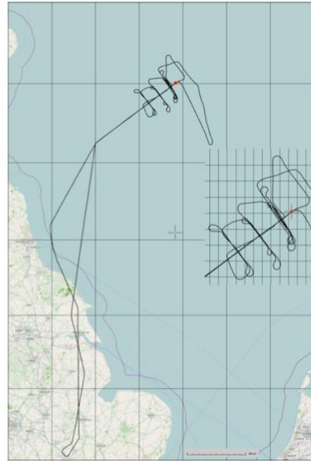
Figure 4.6b (Left): Left Plume measurements of methane made at various heights and distances downwind of the Elgin gas platform, used to then estimate the mass emission strength.
