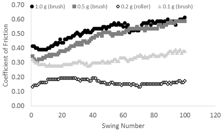
Figure 15 Pendulum tests using different amounts of TORFM and different application methods
