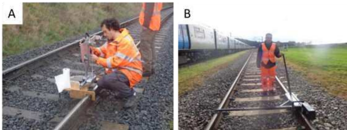
Figure 6 A) Pendulum at SVR, B) Salient Systems tribometer at LM
