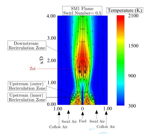
Fig. 8 The predicted structure of SM1 flame.
