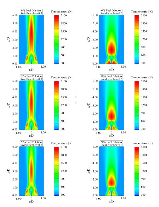
**Fig. 15** The temperature contours for the cases with 0%, 10% and 20% fuel dilution and swirl numbers of 0.3 (left) and 0.6 (right).
