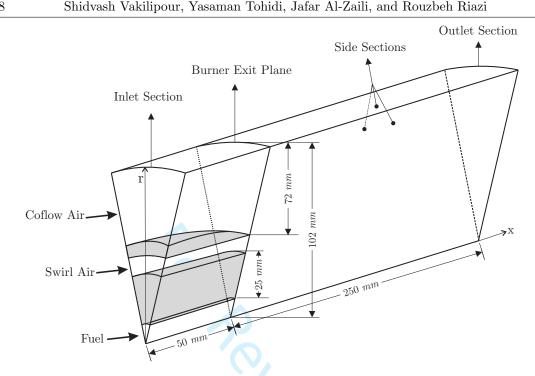
Fig. 2 The configuration of 2-D wedge-type computational domain.
