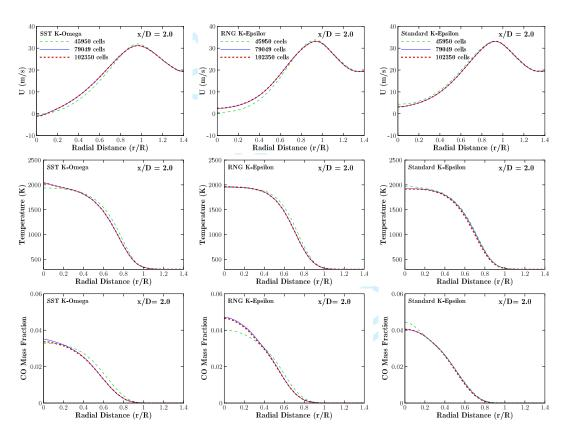
Fig. 3 Grid sensitivity study of the predicted axial velocity, temperature, and CO mass fraction for three distinct turbulence models.
