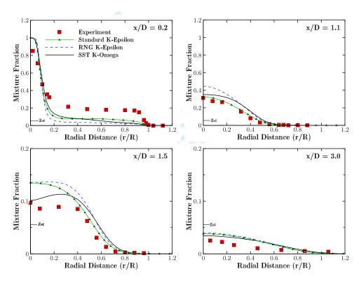
Fig. 5 Radial profile of predicted mixture fraction compared with measurements at different axial locations.
