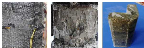
(a) CFRP cloth rupture (b) Crush of concrete core (c) RPC patch
