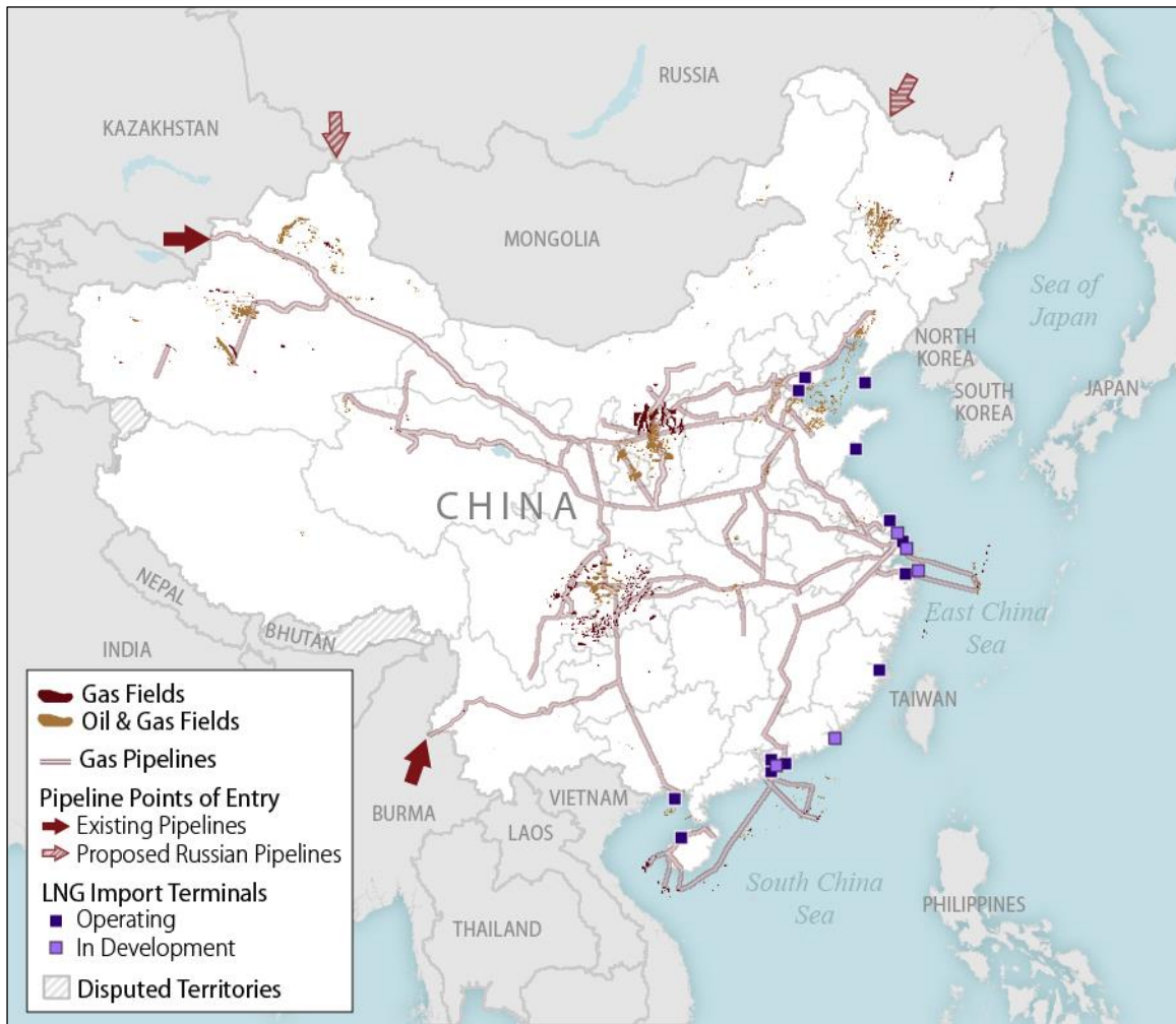
Figure 2: China's Natural Gas Resources and Infrastructure Assets (Source Ratner et al. 2016)
