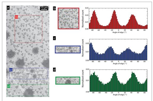
Figure 3. (a) SEM image of copper foil with triangular h-BN islands. Panels (b)–(d) show directionality analysis of the sections of image as indicated, revealing the preferred orientation of the triangular islands in each.
