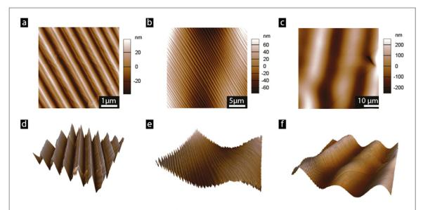
**Figure 4.** AFM topography images of h-BN on copper foil, the h-BN here fully covers the graphene surface. Panels (d)–(f) are the corresponding three-dimensional views of the surface topographies shown in (a)–(c).
