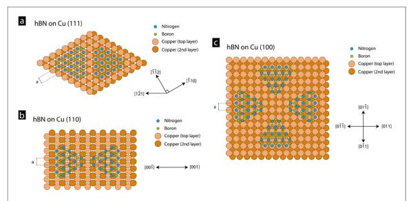
**Figure 6.** Atomic structure of monolayer h-BN on different orientations of copper surface, showing the top two atomic layers of each copper surface orientation. Panel (a) is for h-BN on Cu(111), (b) h-BN on Cu(110), and (c) h-BN on Cu(100).
