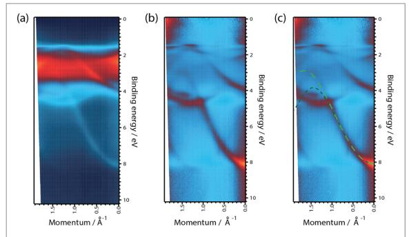
**Figure 8.** ARPES data from a full coverage h-BN sample. Left; raw image, centre; momentum distribution curve (MDC) normalized image, right; MDC normalized image with the dispersions of a tight-binding model for h-BN overlaid in green; the tight binding dispersion in the  $\Gamma M$  direction is the darker green line with shorter dashes, and in the  $\Gamma K$  direction is the lighter green line with longer dashes.
