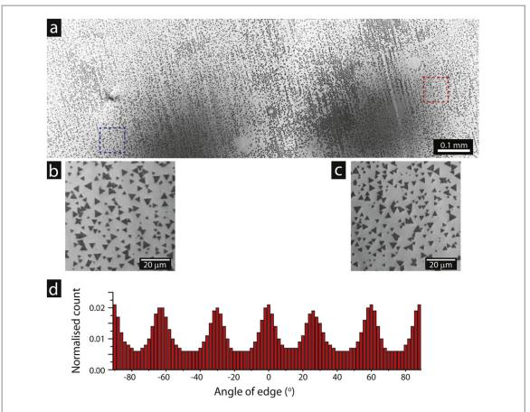
**Figure 7.** (a) Low magnification, high pixel density SEM image of h-BN islands on a single millimetre sized vicinal Cu(100) region of copper foil. Panels (b) and (c) show magnified sections of the image with clearly resolved triangular h-BN islands. The directionality histogram in (d) was obtained from the entire image and clearly shows peaks in edge orientation separated by 30°.
