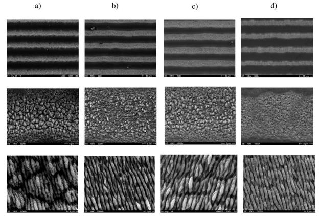
A-1.2: Titanium surfaces fabricated in air using femtosecond laser. Figures represented a) TTL1-Air, b) TTL2-Air, c) TTL3-Air and d) TTL4-Air.
