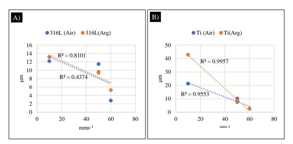
Figure 6-5 Correlation between A) max height surface, *Sz* and laser scan speed (mms<sup>-1</sup>) on 316L (air) and 316L (argon), B) max height surface, *Sz* and laser scan speed (mms<sup>-1</sup>) on Ti6Al4V (air) and Ti6Al4V (argon).
