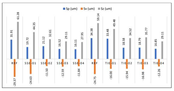
Figure 5-4 Graph of height parameter on 316L and Ti6Al4V with respect to maximum height surface parameter, SP (max peak height), Sv (max valley depth) and Sz (max height of surface)
