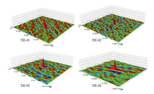
Figure 5-9 ACF on WEDM titanium specimen
