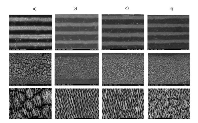
A-1.0: Stainless steel surfaces fabricated in air using femtosecond laser. Figures represented a) SSL-01-Air, b) SSL-02-Air, c) SSL-03-Air and d) SSL-04-Air.
