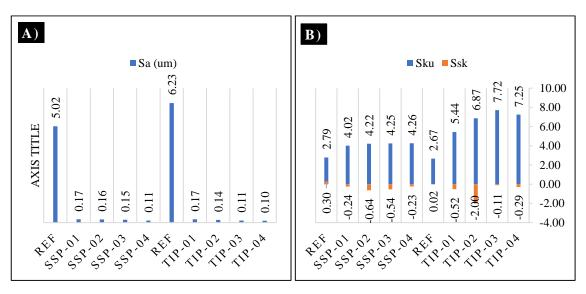
Figure 4-1 Graph of the height parameters on 316L and Ti6Al4V with respect to A) *Sa* and *Sq*, B) *Sku* and *Ssk*
