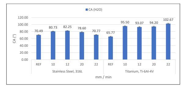
Figure 5-10 A graph of contact angle measurement on EDM specimen
