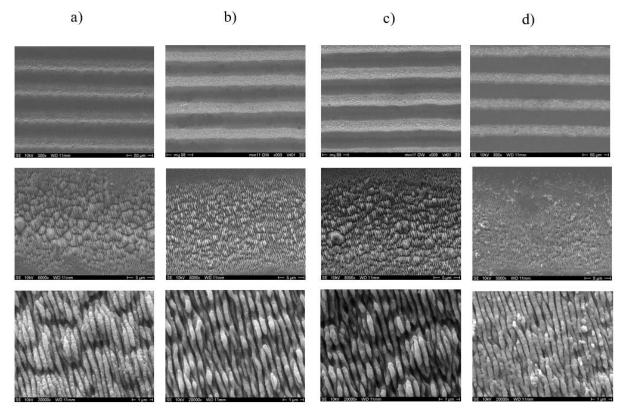
A-1.1: Stainless steel surfaces fabricated in argon using femtosecond laser. Figures represented a) SSL-01-AR, b) SSL-02-AR, c) SSL-03-AR and d) SSL-04-AR
