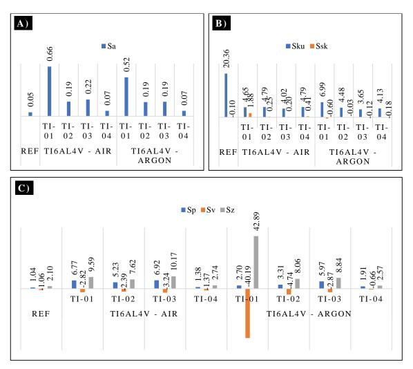
Figure 6-3 Graph of height parameter on 316L and Ti6Al4V with respect to a) *Sa* and *Sq*, b) *Sku* and *Ssk* and c) *Sp* (max peak height), *Sv* (max valley depth) and *Sz* (max height of surface)
