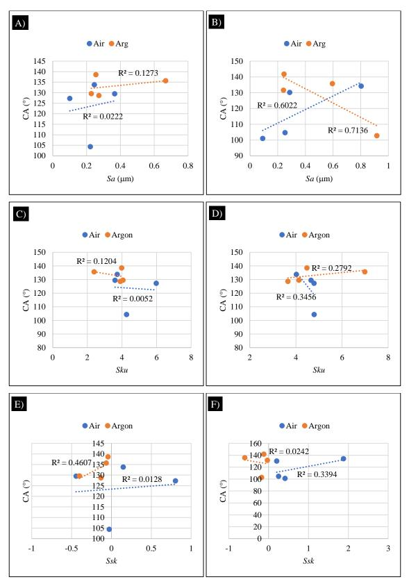
Figure 6-9 Correlation between contact angle and A) average roughness, Sa on 316L C) surfaces kurtosis, Sku on 316L, E) surface skewness, Ssk on 316L, B) average roughness, Sa on Ti6Al4V, D) surface kurtosis, Sku, F) surface skewness, Ssk.
