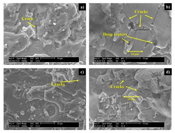
Figure 5-2 WEDM titanium morphology a) TIE-01 (10mm/min), b) TIE-02 (12mm/min), TIE-03 (20mm/min) and d) TIE-04 (22mm/min)
