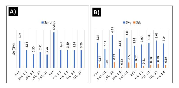
Figure 5-3 Graph of the height parameters on 316L and Ti6Al4V with respect to A) *Sa* and *Sq*, B) *Sku* and *Ssk*
