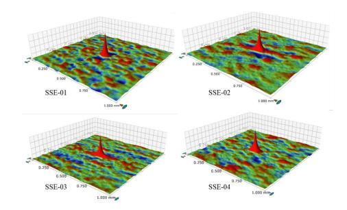
Figure 5-8 ACF on WEDM stainless-steel specimen
