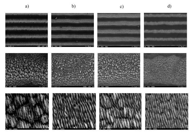
A-1.2: Titanium surfaces fabricated in argon using femtosecond laser. Figures represented a) TTL1-Air, b) TTL2-Air, c) TTL3-Air and d) TTL4-Air.
