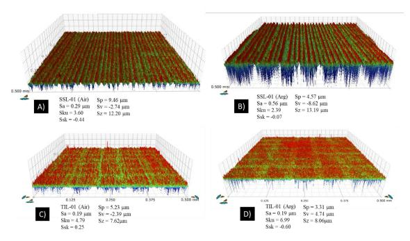
Figure 6-6 3D optical profilometry images on SSL-01 (Air) and SSL-01 (Ar)
