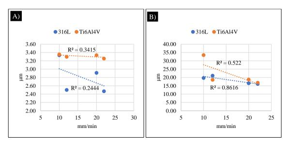
Figure 5-6 Correlations between a) average roughness, *Sa* (µm) and machine feed rate (mm/min) b) maximum height surfaces, *Sz* (µm) and machine feed rate (mm/min) on WEDM stainless-steel and titanium.  $R^2 > 0.7$  indicated strong correlation,  $R^2 = 0.5 - 0.69$  represented moderate correlation and  $R^2 = 0.49 - 0.3$  poorly correlated and  $R^2 < 0.29$  provided no correlation.
