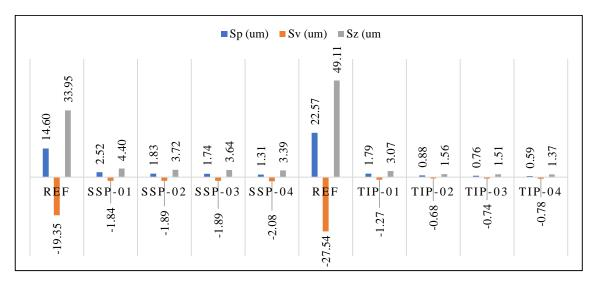
Figure 4-2 Graph of the height parameters on 316L and Ti6Al4V with respect to height surfaces parameter, SP (max peak height), Sv (max valley depth) and Sz (max height of surface)
