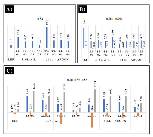
Figure 6-2 Graph of height parameter on 316L and Ti6Al4V with respect to a) *Sa* and *Sq*, b) *Sku* and *Ssk* and c) *Sp* (max peak height), *Sv* (max valley depth) and *Sz* (max height of surface)
