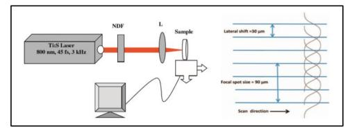
Figure 2-1: Schematic set up of laser fabrication of bioactive glass where the laser beam is passed through the neutral density filter (NDF) and lens (L = 5 cm focal lengths) before hitting the sample on the computer-controlled X-Y stages.
