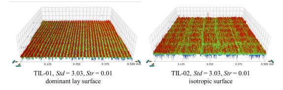
Figure 6-7 The difference between dominant lay surface and isotropic surface of Ti6Al4V
