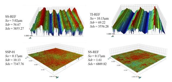
Figure 4-3 Bruker images of polished stainless-steel and titanium
