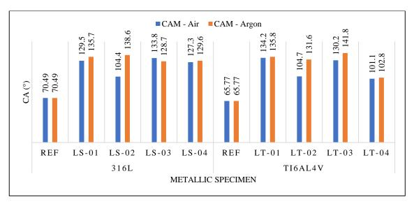
Figure 6-8 Graph of water contact angle on laser-assisted on 316L and Ti6Al4V
