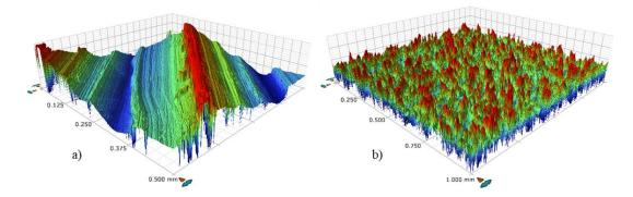
Figure 5-7 3D optical profilometry images for a) Ti6Al4V with Std = -81.23, Str = 0.10and b) Ti6Al4V with Std = n/a, Str = 0.85
