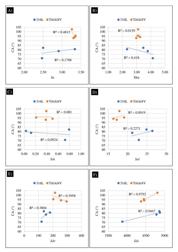
Figure 5-11 The correlation between a) average roughness, Sa b) kurtosis, Sku c) skewness, Ssk d) auto-correlation length, Sal e) developed interfacial area ratio, Sdr h) summit density, Sds with water contact angle on 316L and Ti6Al4V specimens.
