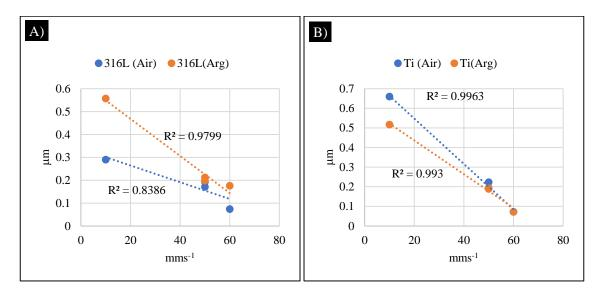
Figure 6-4 Correlation between A) average roughness, *Sa* and laser scan speed (mms<sup>-1</sup>) on 316L (air) and 316L (argon), B) average roughness, *Sa* and laser scan speed (mms<sup>-1</sup>) on Ti6Al4V (air) and Ti6Al4V (argon)..
