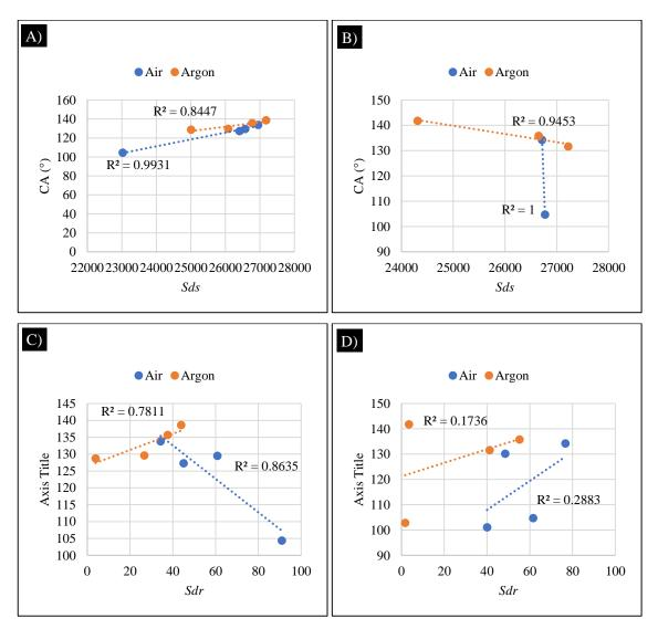
Figure 6-10 Correlation between contact angle and A) summit density, *Sds*, C) developed interfacial area ratio, *Sdr* on 316L, B) summit density, *Sds*, D) developed interfacial area ratio, *Sdr* on Ti6Al4V.
