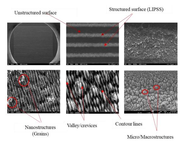
Figure 6-1 Images for the titanium that have undergone femto-second irradiation techniques showing all the available features on the modified surfaces viewed with SEM.
