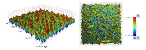
Figure 5-5 3D optical profilometry for TIE-02 with  $Sa = 3.30 \ \mu\text{m}$ , Sku = 3.34, Ssk = 0.38, SP = 33.48, Sv = -15.99 and Sz = 49.48
