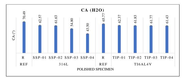
Figure 4-8 Graph of contact angle measurement on metallic polished specimen
