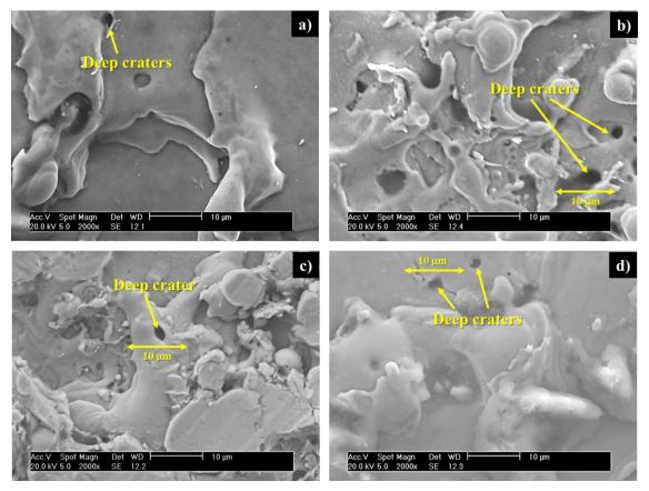
Figure 5-1 WEDM stainless-steel morphology a) SSE-01 (10mm/min), b) SSE-02 (12mm/min), SSE-03 (20mm/min) and d) SSE-04 (22mm/min)
