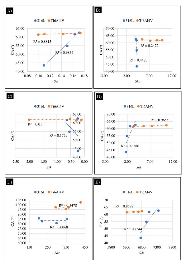
Figure 4-9 Correlation between a), average roughness, *Sa* b) kurtosis, *Sku* c) skewness, *Ssk* d) auto-correlation length, *Sal* e) developed interfacial area ratio. *Sdr* h) summit density, *Sds* with water contact angle on 316L and Ti6Al4V specimen.
