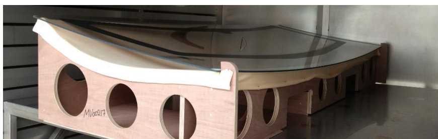
Figure 6.21: A PC flat sheet placed on the forming tool within the oven prior to the thermal forming stage.
