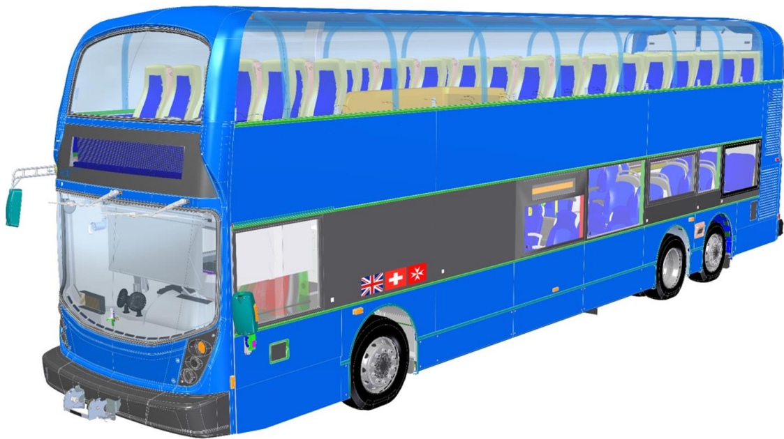
Figure 7.3: A graphical representation of the Enviro500 equipped with the lightweight upper-deck structure.
