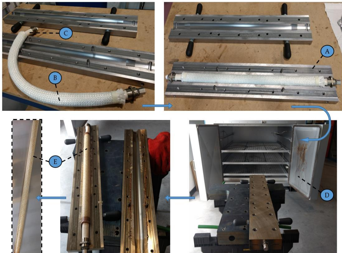
Figure 5.7: An overview of the proposed bladder-assisted consolidation of a braided FR thermoplastic structure. The braided composite preform (B) is supported by an inflatable bladder (C), placed within a simple metal tool (A) and heated within a conventional oven (D) in order to achieve the final consolidated component (E)
