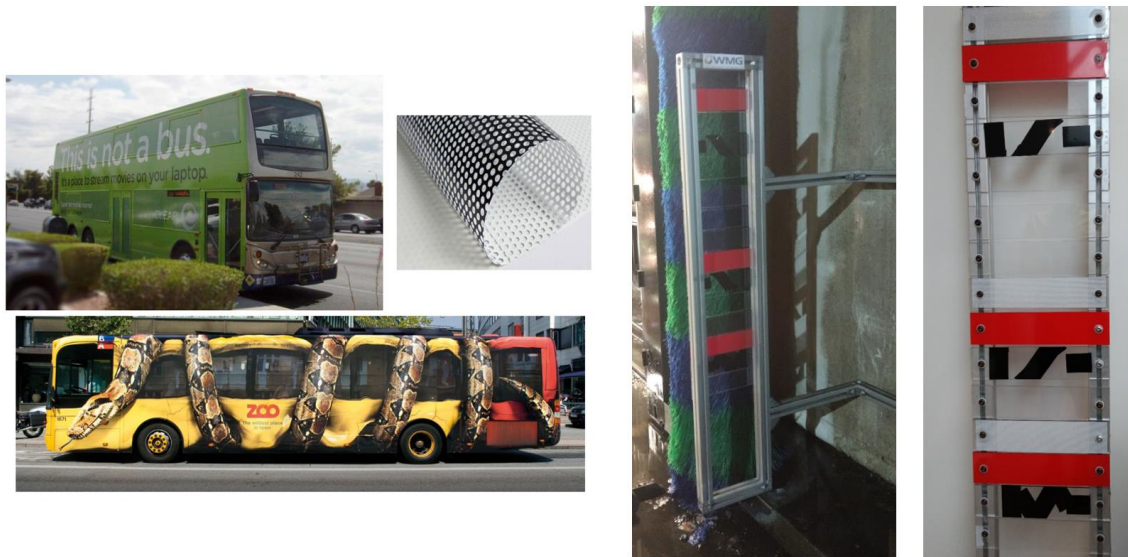
Figure 6.15: Right: the utilisation of see-through adhesive films on buses. PC panels covered with adhesive films – before (middle) and after (right) the bus-wash exposure testing.
