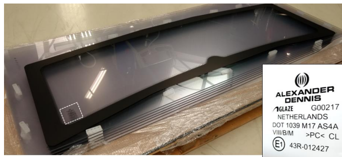
Figure 6.20: The flat sheets following the silk-screen printing process and detail of required markings.
