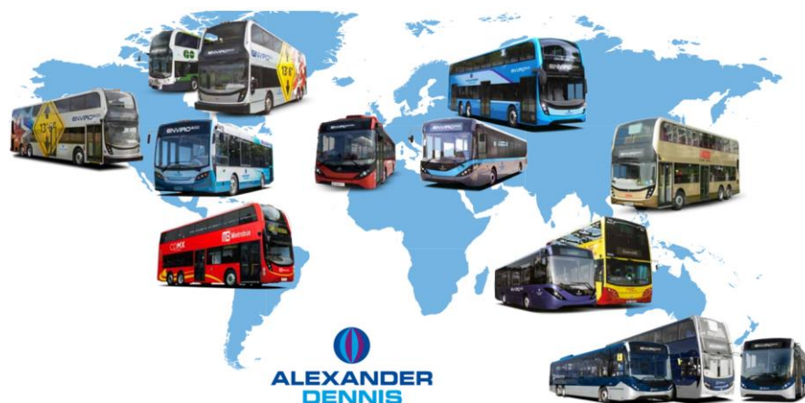
Figure 3.2: ADL's range of low floor buses are based on three different platforms; two-axle single-deck bus (Enviro200), two-axle double-decker bus (Enviro400) and triple-axle double-decker bus (Enviro500), reproduced from [97].
