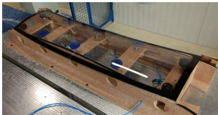
Figure 6.23: The final manufacturing stage consists of machining the panel on a five-axis milling machine.
