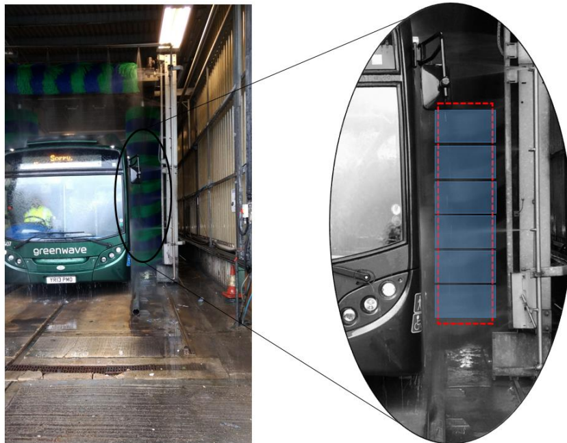
Figure 6.8: Proposal of testing concept: Test samples to be mounted onto a purpose built frame that would allow the test samples to be exposed to the bus-wash brushes whenever the bus-wash is in operation.
