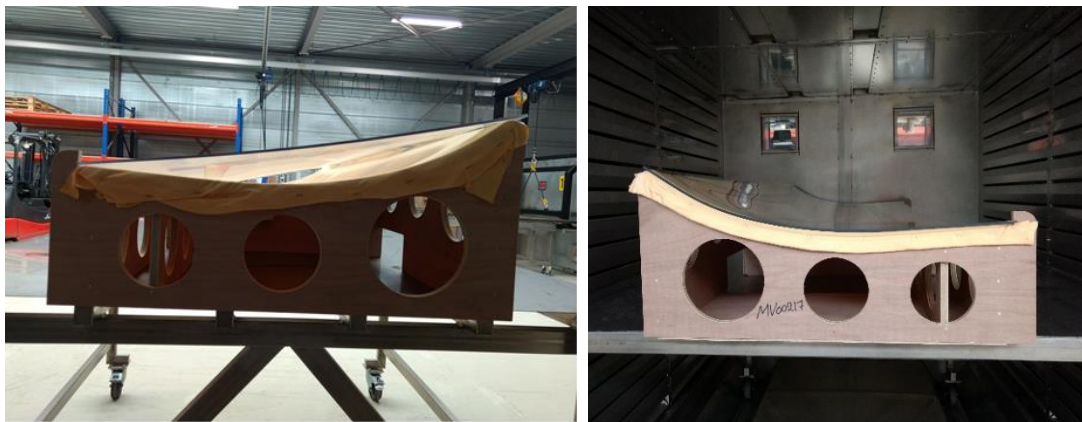
Figure 6.19: The flat sheet of PC placed on the forming tool (left) and the curved panel following the curing cycle (right).
