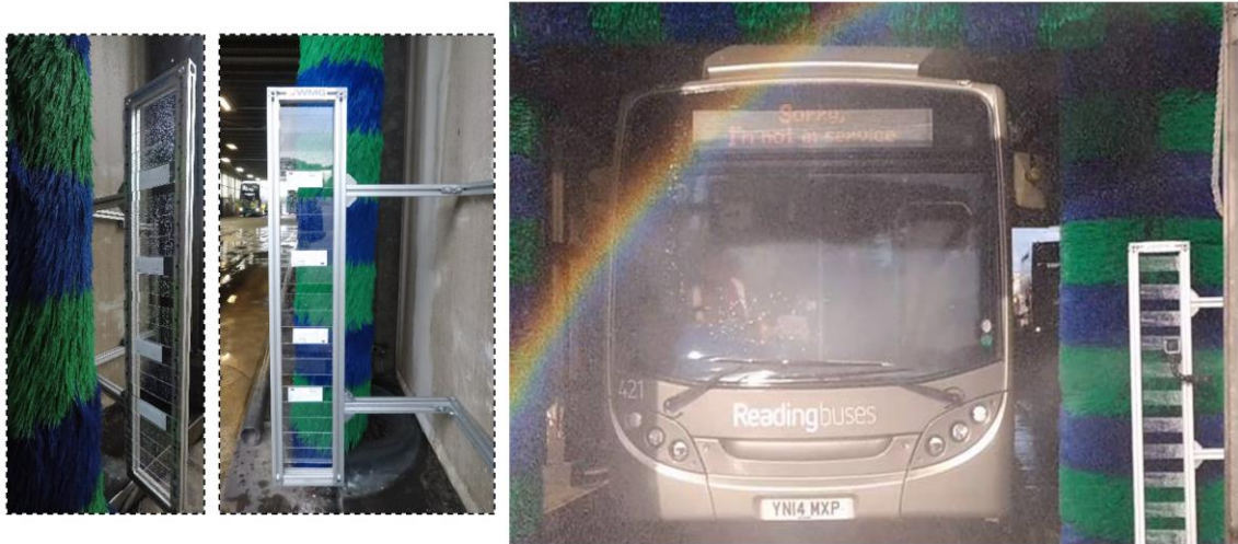
Figure 6.10: Frame with test samples mounted on the bus-wash at Reading buses depot. Left and middle: Side view of the frame with the test panels mounted. Right: Test samples exposed to the brush washing action whilst a bus is undergoing the automatic wash cycle.
