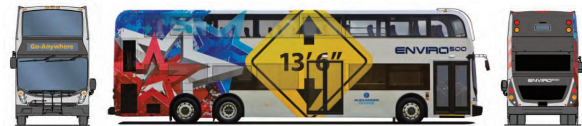
Figure 4.1: ADL Enviro500: 13 m long, 3-axle bus with 26,500 kg GVW, reproduced from [117].
