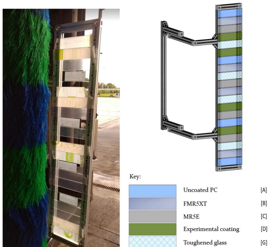
Figure 6.12: Set-up for the main testing phase. Four repeats of three different coated PC panels, an uncoated PC panel and a control glass panel were randomly placed on the frame.
