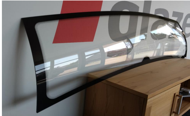
Figure 6.25: The finished PC glazing panel – ready for installation onto buses for in-service trials.
