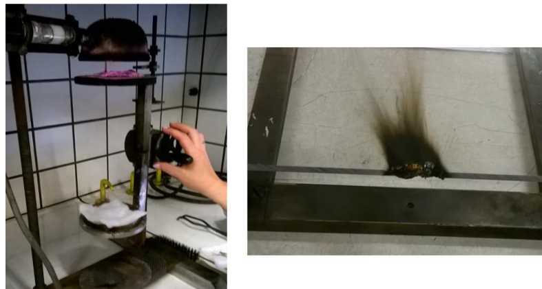
Figure 6.16: Left: Drip-test being carried out on coated PC samples. Right: Results of the vertical burn test. All tested specimens successfully and robustly passed the tests. Tests carried out as specified by Annex 7 and 8 of ECE Add.117, R118 [121].
