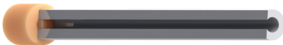
Figure 4.25: Static coating procedure with plug at column end
