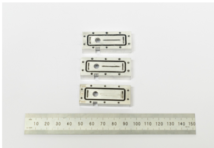
Figure 5.7: Design-3 ionisation chamber with 0.3, 0.1, 0.05 mm channel depth and split sample path
