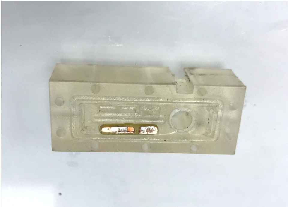
Figure 5.12: 3D manufactured ionisation chamber with exposed slots for electrode pads
