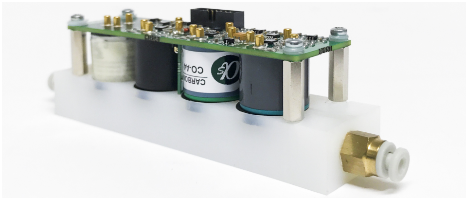
Figure 3.14: PID, CO, NO 2 and H 2 S and the AFE housed in a gas hood.
