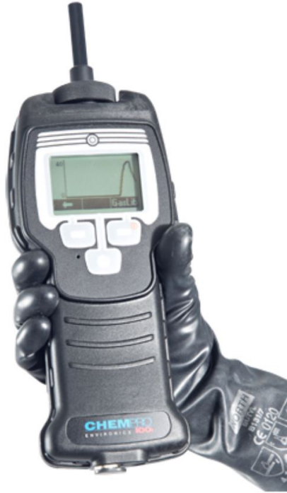
Figure 2.11: The Chempro 100i using aADT IMS drift tube [65].
