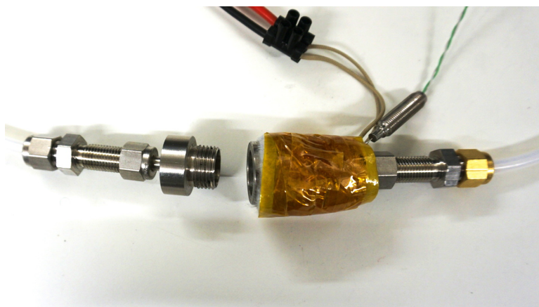
Figure 4.5: Assembled Concept-1 thermal desorber for ACC
