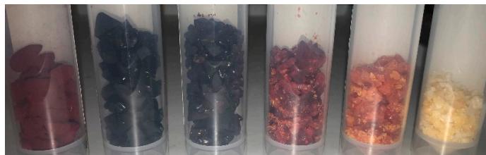
Figure 3. RMF gels prepared under acidic conditions with varying melamine content: from left to right [M] = 0%, 20%, 40%, 70%, 90%, and 100%.
