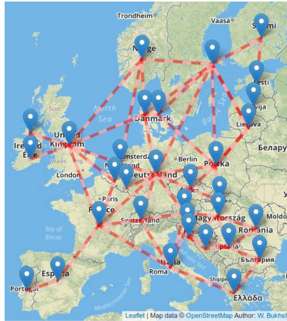
Figure 1: A representative European electricity transmission network. Each country is represented by at least a node. The Net Transfer Capacities (NTC) are used to model the capacities of the links between the nodes and are obtained from the Ten Year Network Development Plan (TYNDP).
