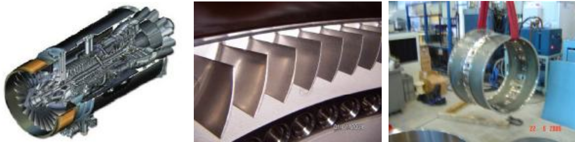
(a). More than 90% thin-walled parts. (b). Asymmetric-open-blades. (c). Axisymmetric-closed-casing. Figure-1. A typical aero-engine construction
