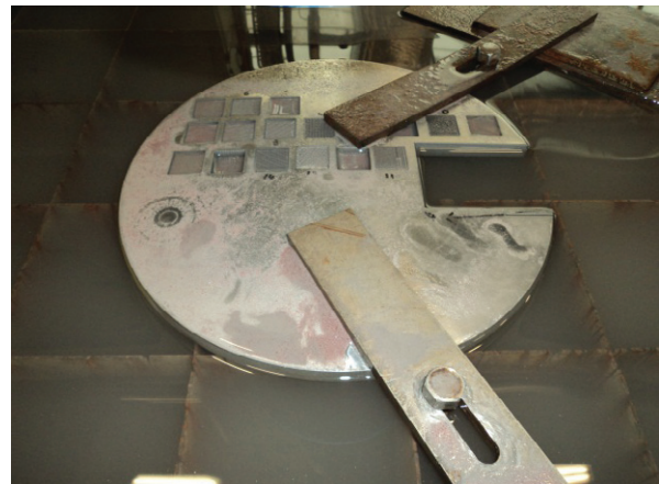
Fig. 2 Experimental set-up; the inconel plate is clamed onto the AWJ table and pockets are cut
