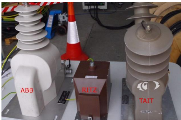
Figure 2: 11 kV voltage transformers used in testing at PNDC
