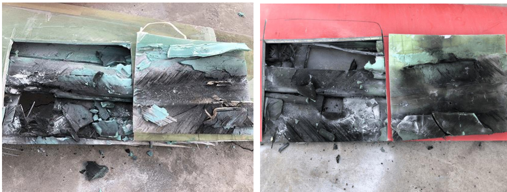
(a) arc path I (b) arc path II Fig. 7 Inside damage of the blade with different arc paths
