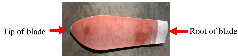
Fig. 3 5m long specimen cut from the real blade.
