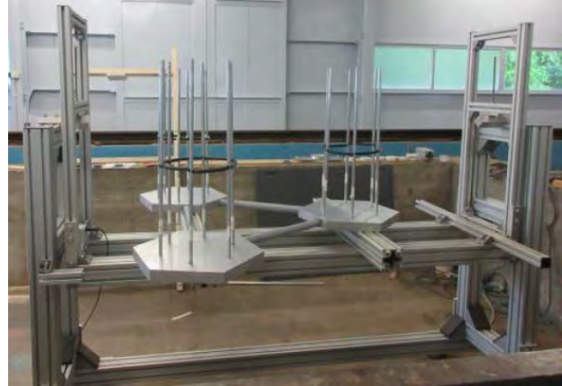
Figure 3 Test model ballast keel mass properties being tested in the Pendulum Swing Device at KHL, Glasgow.
