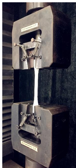
Fig. 5. The tensile machine and specimens under testing.
