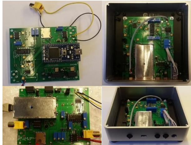
Figure 3.52. Illustration of iSim PCB assembly iteration and enclosure testing.
