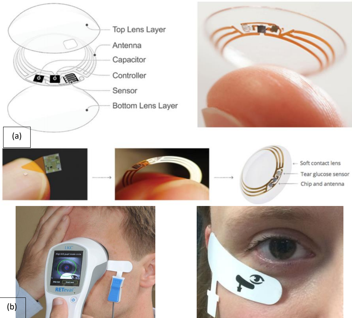
Figure 2.26. (a) Contact lens sensor developed by Google and Novartis (called “ smart lens technology ”). This product has an embedded glucose biosensor embedded into a hydrogel matrix that senses the glucose level in the tear and transfers the data wirelessly using the embedded controller and antenna to a nearby computer or phone [296]. Several patents granted to Google, Johnson and Johnson Vision Care Inc and others on continuous monitoring of the tear glucose from 2009 to 2014 [301]. Such a contact lens system cannot currently be used in electroretinography applications. However, with the trend of increasing miniaturisation of devices and systems, it is becoming increasingly possible to make even smaller, multifunctional, higher speed devices that can potentially provide many of the critical features requirements of a laboratory ERG instrumentation. (b) Left: The first handheld system (RETeval LKC Technologies) developed and commercially made available for VEP, ERG and flicker examinations using skin electrodes without the requirement for pupil dilation and administration of anaesthesia. Right: placement of the device sensor strip, the setup requires no skin preparation. The effect of position of this electrode array is investigated by Hobby and Kozareva et al (2018)[299].
