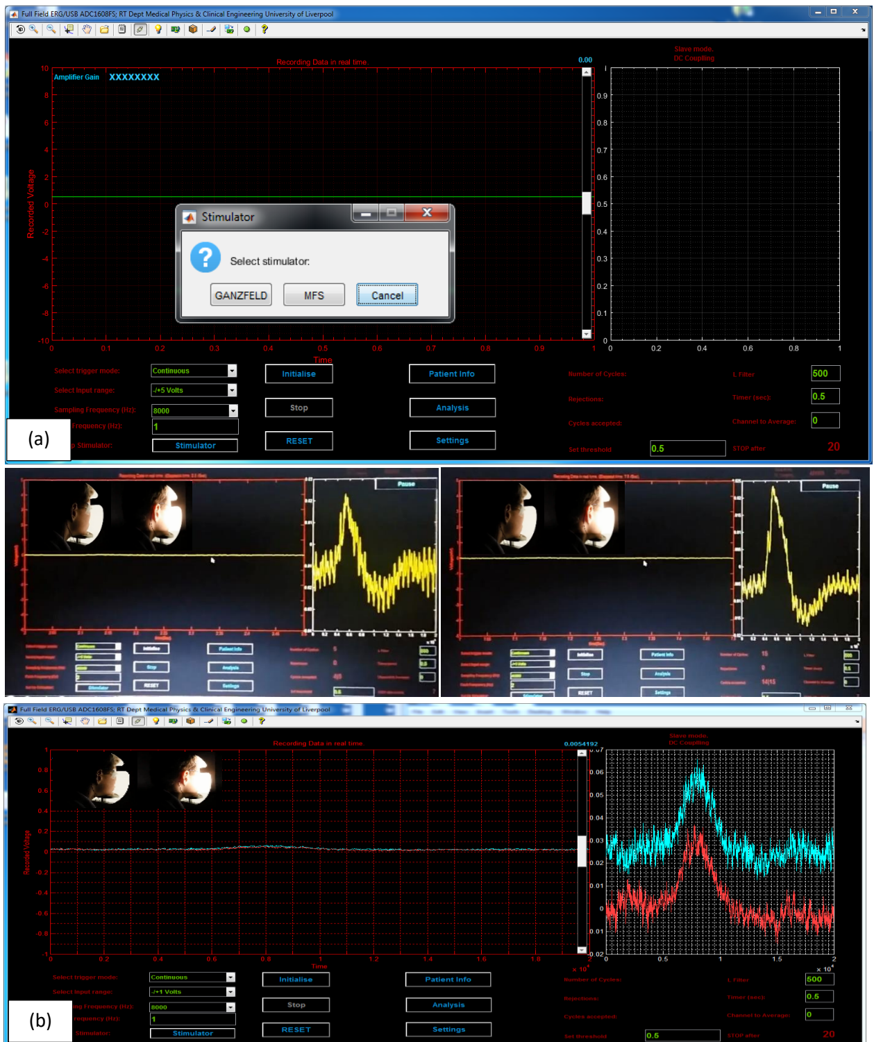
Figure 3.30. (a) Illustration of the MATLAB® GUI to communicate with bio-amplifier and stimulator. (a) shows the interface and a popup dialogue box that allows user to select the stimulator type. (b) Illustration of bio-amplifier main GUI during study subject test run using Ganzfeld Roland system while performing flash stimulation of -25 dB below ISCEV specified standard flash intensity of 3 cd.s.m -2 . There are two plot areas, the one on the left is a plot of collected data filtered at 500 Hz low-pass corner frequency with no other signal processing and the one on the right which demonstrates the signal average in real-time. The pause button on the top right corner is only visible when the system is running and provides a mechanism to pause signal averaging and storing while still reading and plotting the biological waveform. The artefact auto-rejection mechanism is active when collecting data, the operator will have access to raw data including all recorded artefacts. Figure (b) also demonstrates recording from both eyes through activating both bio-amplifier channels.
