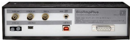
Figure 3.28. (a) Illustration of the clinical/study setup and the required connections. As well system being powered through an isolation transformer block allowing the measurement units and the subject connected to it to float for safety and noise reduction purposes. (b) Illustration of designed and developed bio-amplifier showing input and output terminals including amplifier's two recording channels, optical trigger in/out, USB terminal, other exposed input and out digital pins (DIO lines) as well as MCC onboard LED. The gain switch between a gain of unity and 5000 is also demonstrated. (c) Illustrates the initial signal channel bio-amplifier prior to advancing to development of a two-channel bio-amplifier with higher specification.
