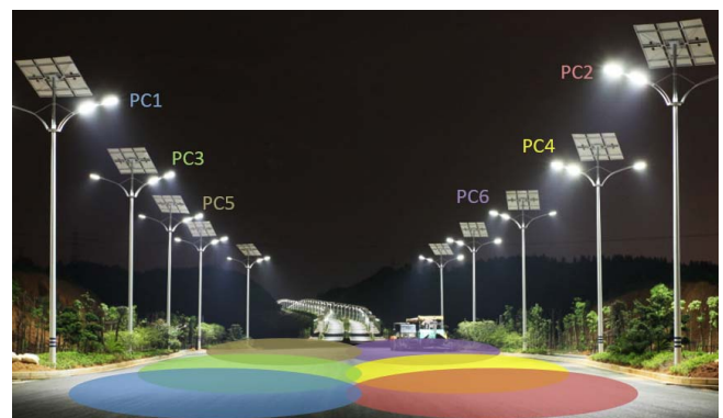
Fig. 1. The illustrative scenario of the 5G coverage area using the proposed PC base station.
