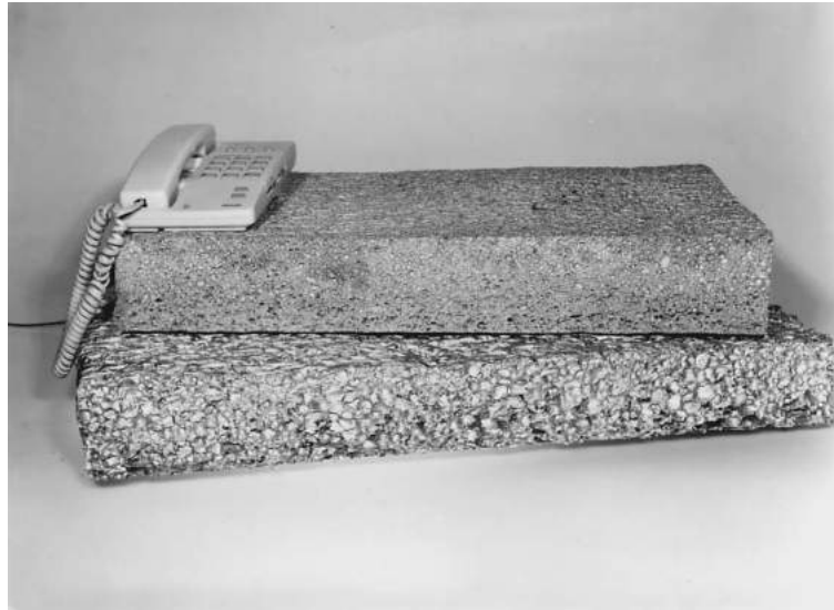
Figure 2.1: Aluminium slabs of two different porosities and cell sizes produced by the gas injection method. (Banhart 2001).
