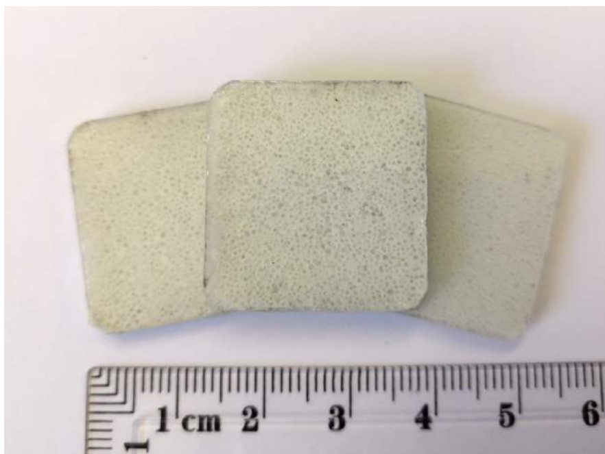
Figure 3.8: Typical porous glass samples produced by the SDP process.
