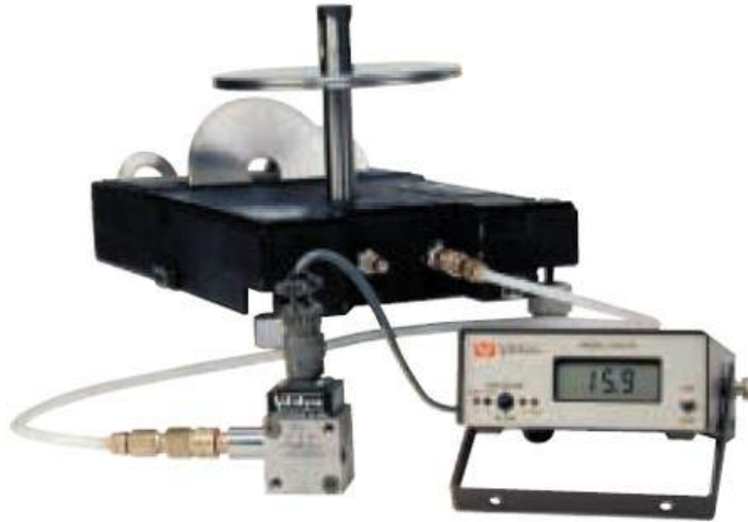
Figure 3.16: The calibration system for the pressure transducer.
