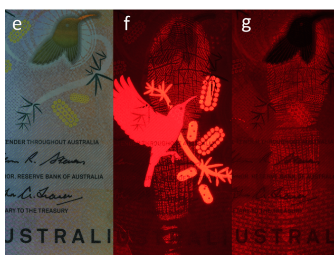
Figure 3. (a,c,e) Unilluminated and (b,d,f) illuminated at 350 nm and (g) 450 nm charged latent fingermarks (one female donor) deposited on Australian polymer banknote. The illuminated marks were pictured through a deep red filter. The marks were shaken at 20 rpm for 20 min in a MPA-coated CIS-ZS QDs solution. See ESI+ and Table S1 for the photography details.
