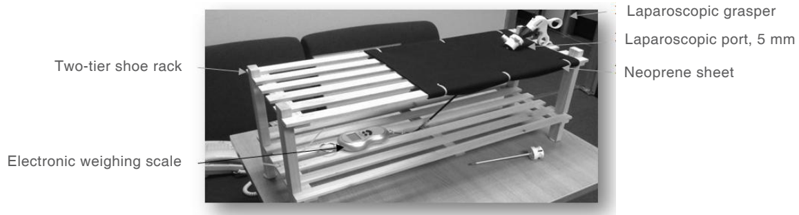
Figure 3. Home-made laparoscopic task setup
