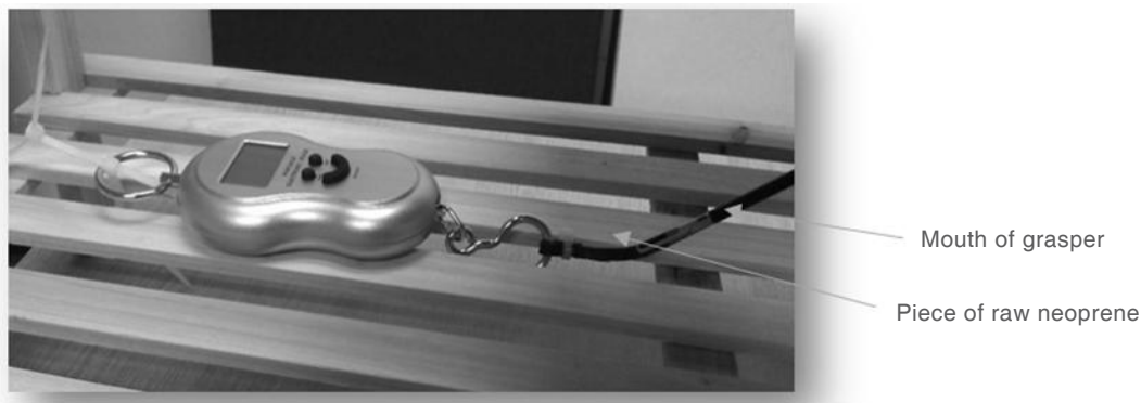
Figure 4. Mouth of grasper was locked to hold the piece of neoprene
