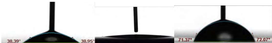
FIGURE 5.6: Water droplet on bare (left), hydroxylated (center) and silanized (right) silicon. The change in shape of the droplet demonstrates surface modification. The hydroxylated silicon is very hydrophobic, therefore the contact angle was very small ( \sim 5^\circ ) and not easily detected by the software at the moment when the image was taken
