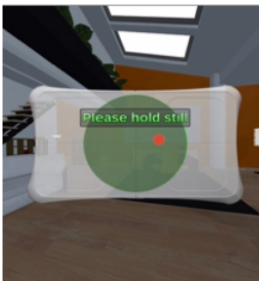
Figure 6. The visual calibration screen shown to the participants prior to each trial. An example of the image participants viewed pre-trial through the Oculus Rift headset. The red dot represents the participants COP. The participants were required to keep their COP within the larger green circle, aiming for the central cross hair, prior to each trial to ensure they were stable. The calibration phase gave the individuals visual feedback regarding their balance to ensure they were maintaining their postural equilibrium prior to all the trials. The trial would not begin unless the individuals COP was held within the larger green circle for 3 seconds, for which the individuals viewed a visual countdown screen.
