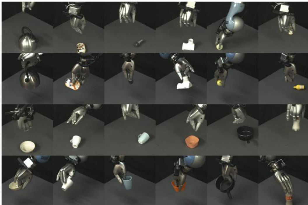
Figure 3.15: Examples of grasps generated by the generative model (GM, 1 st and 3 rd row) and the generative-evaluative model (GEA, 2 nd and 4 th row) on paired trials. The first five columns show some of the 15 cases where the GEA model succeeds but GM fails. The far right-hand column shows 2 of the 5 converse cases.
