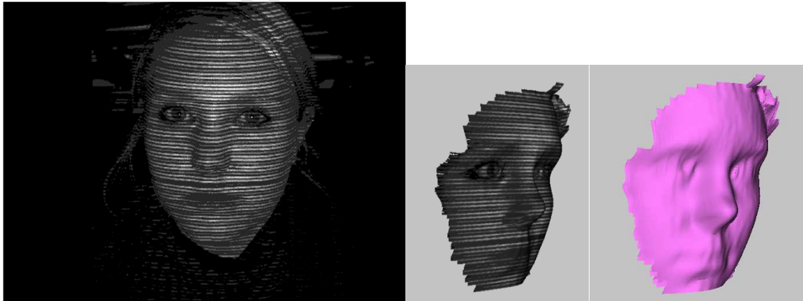
(left) 2D decompressed Face1 image with RMSE=11.5, (middle and right) converted the 2D Face1 image to 3D surface by the GMPR method at compressed size =18.1 KB.
