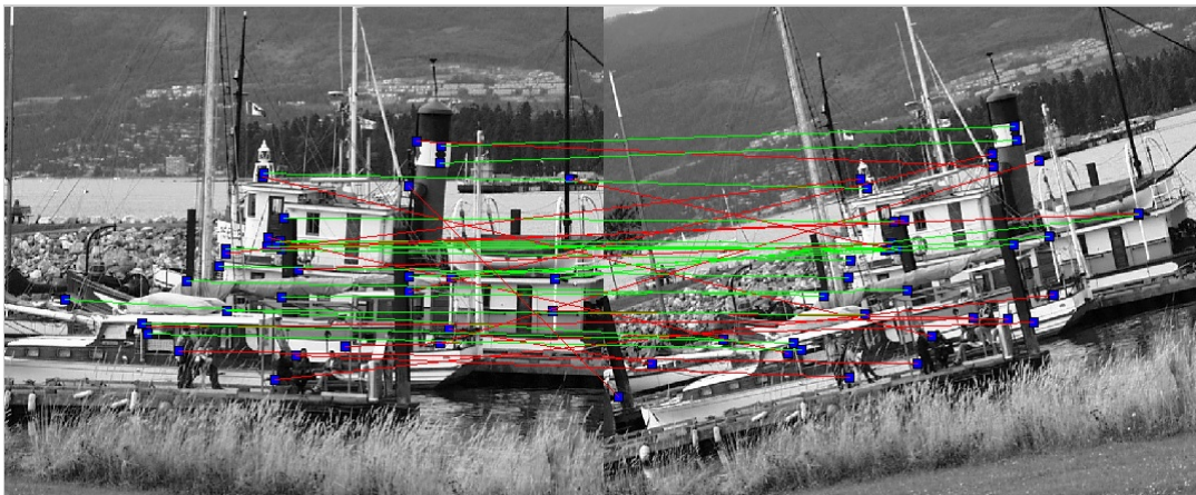
(a) Points detected by SURF method and matched by FastBipartite algorithm
