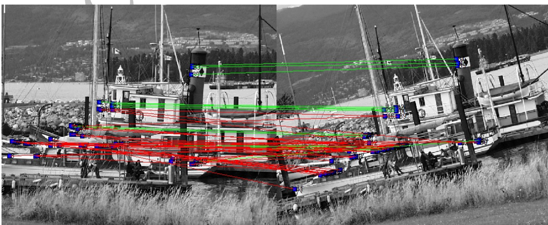
(c) Points detected by SIFT method and matched by MatchFeatures Matlab function
