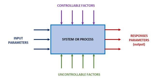
Figure 2.4. Diagram of the design of experiments approach
