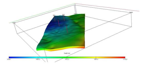
Figure 4.1. Structural map of the field with the exploration and appraisal wells
