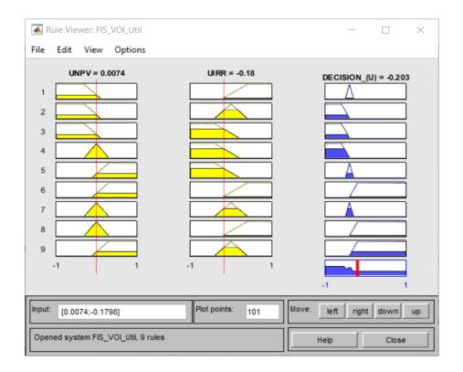
Figure A1.9. FIS evaluation for the data acquisition alternative: extended well test fuzzy data
