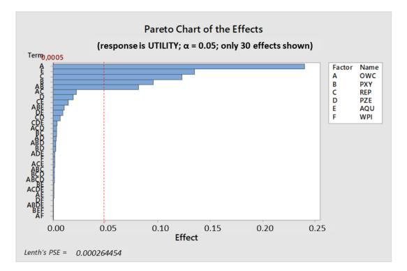
Figure 4.5. Pareto chart of the effects of the parameters, with a significance level of 0.05
