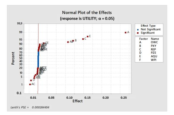
Figure 4.6. Normal plot of the effects of parameters, with a significance level of 0.05
