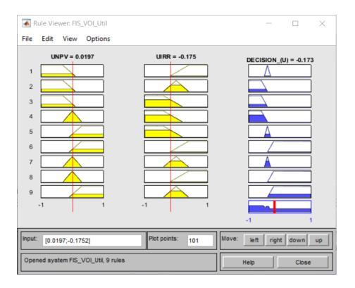
Figure A1.8. FIS evaluation for the data acquisition alternative: extended well test
