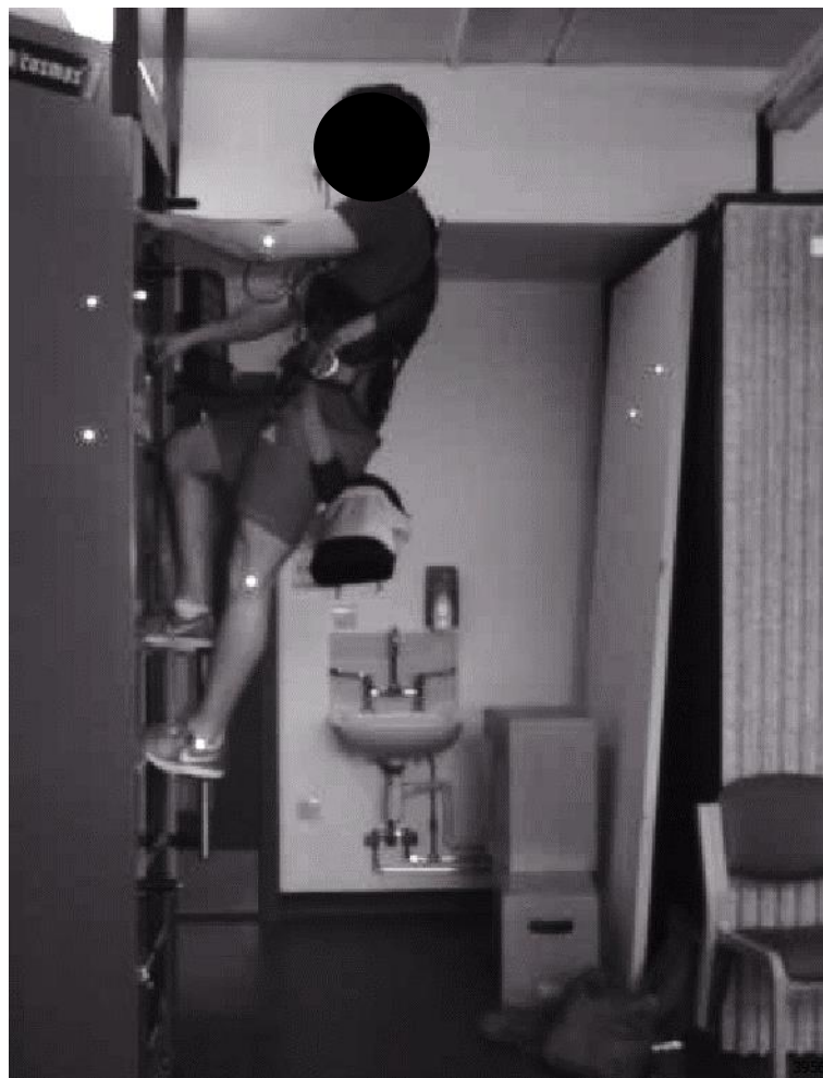
Figure 7.3. Example of external climbing load attached
