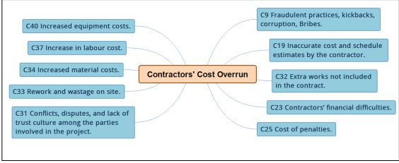
Figure 41: Direct causes of contractors' cost overrun.
