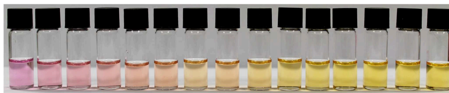
FIGURE 5 | (Top) UV-vis titration of NAz-6-Bpin in THF (0.5 mM) with TBAF. (Bottom) Titration image of NAz-6-Bpin in THF (0.5 mM) with TBAF as a solution in THF. Equivalents of TBAF increase from left to right by 0.1 equivalents, starting at 0 equivalents and reaching 1.4 equivalents.
