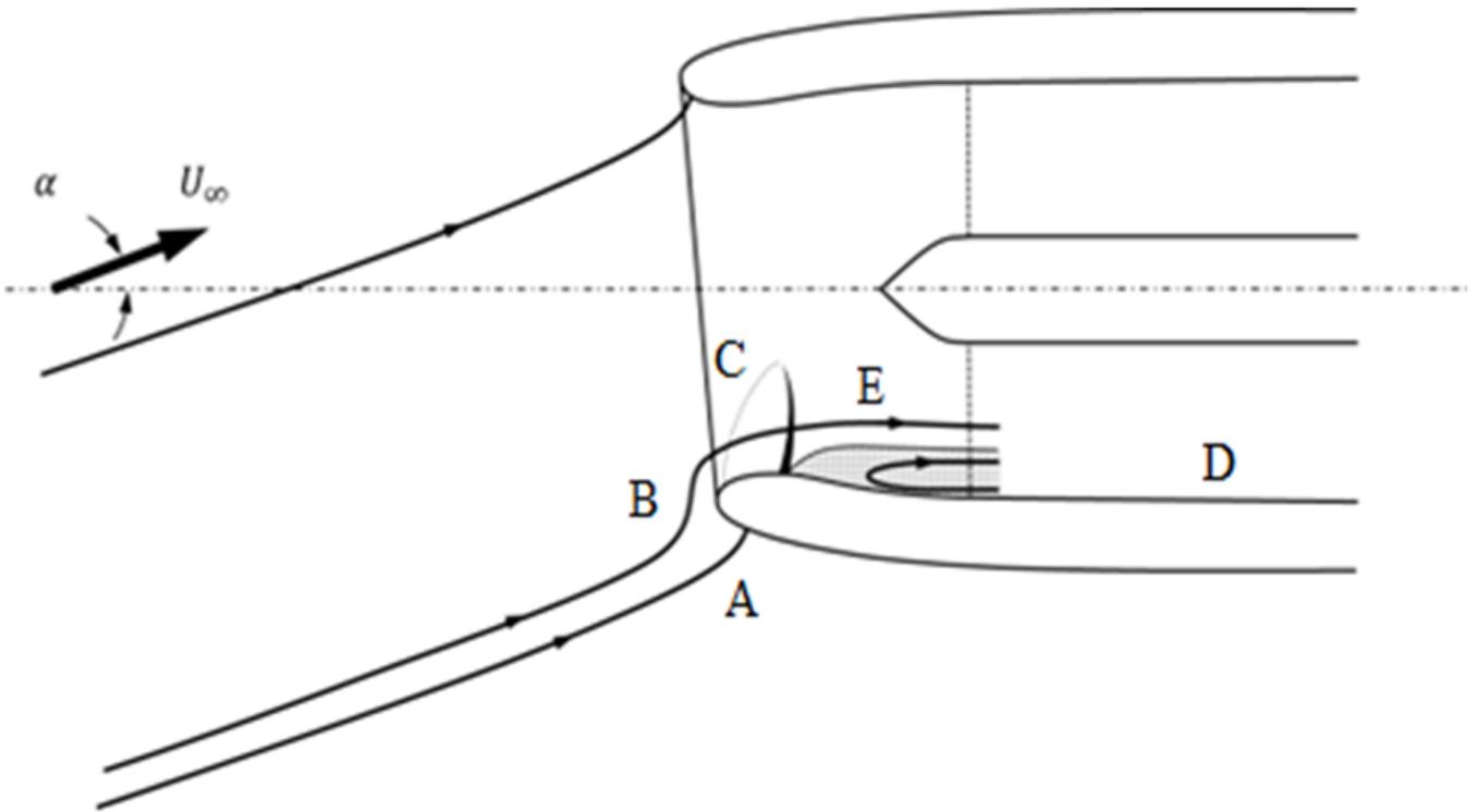
FIGURE 1: Flow arrangement in an intake operating at high incidence.
