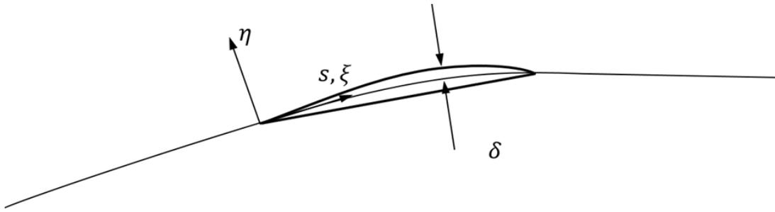
**FIGURE 2:** Curvilinear coordinate system along the blade streamlines.
