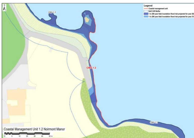
Figure 3: Coastal Flooding and Soft Cliff Buffer Zone at CMU 1.2 Noirmont Manor.
