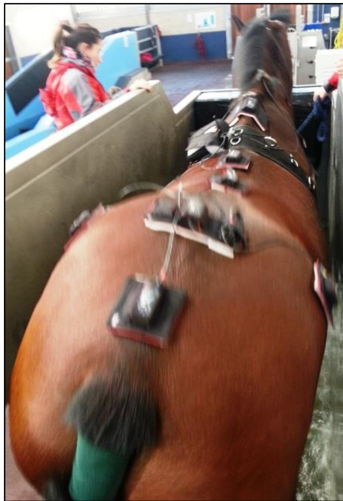
Figure 2.5: A horse on the aqua-treadmill with the Xsens© sensors attached undertaking the set exercise protocol.
