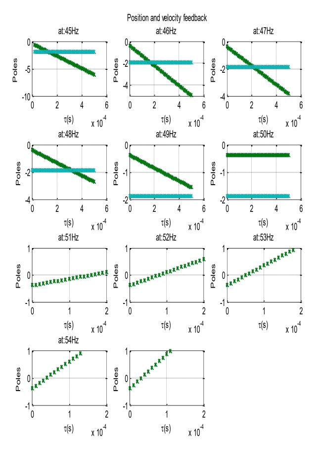
Figure 6-22 System poles variation with position and velocity feedback showing unstable pole after 50Hz
