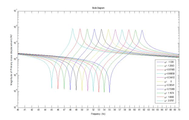
Figure 11-5 Frequency response of the primary mass with acceleration feedback
