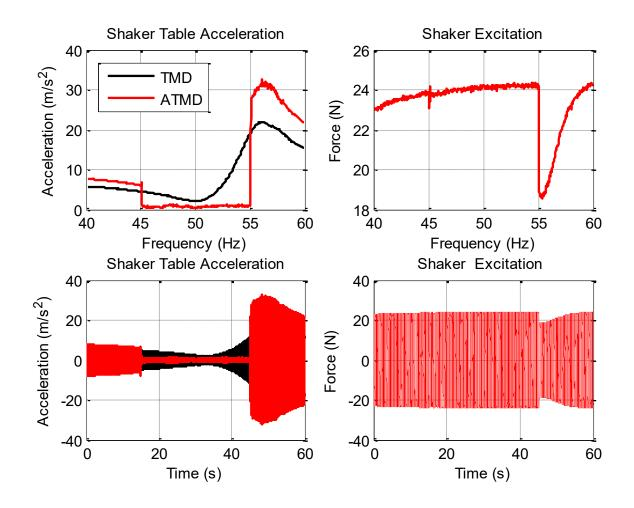
Figure 7-35 Shaker table excitation and acceleration
