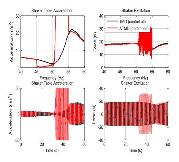
Figure 7-20 Test1: Shaker table excitation and acceleration
