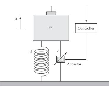
Figure 3-7 Semi-active damping based on manipulating damper properties (Tong, 2014)
