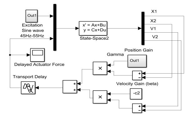
Figure 6-23 SIMULINK model for delayed actuator force with position and velocity feedback
