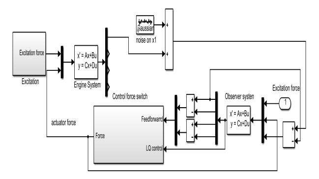
Figure 6-17 State observer with noise
