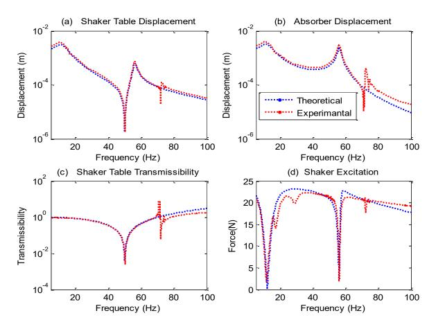
Figure 7-4 Theoretical model results vs experimental results without the VCM
