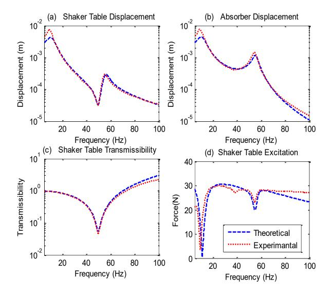
Figure 7-8 Updated theoretical model results vs experimental results with open circuited VCM ( $c_2 = 7 Ns/m$ )
