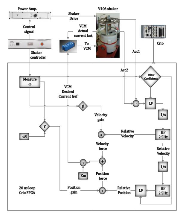
Figure 7-30 Schematic Diagram of the control model of Test 3
