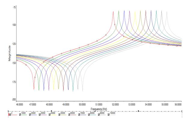
Figure 11-10 Frequency response of the electrical analogous system with electrical charge (Q) feedback
