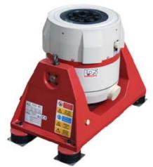
Figure 5-3 Photo of the electromagnetic shaker used in the experiment (Bruel & Kjaer)
