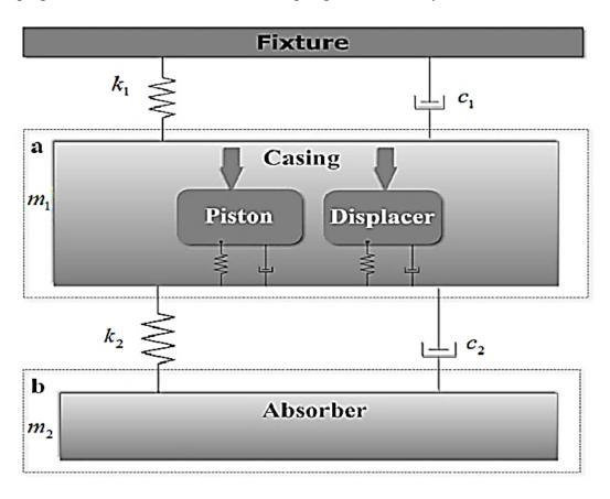
Figure 5-1 Dynamic model of the  $\beta$ -type Stirling engine showing a casing
