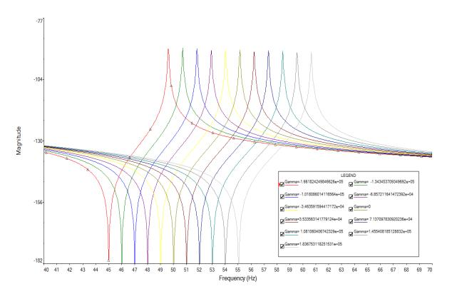
Figure 11-14 Frequency response with charge and negative current feedback gain
