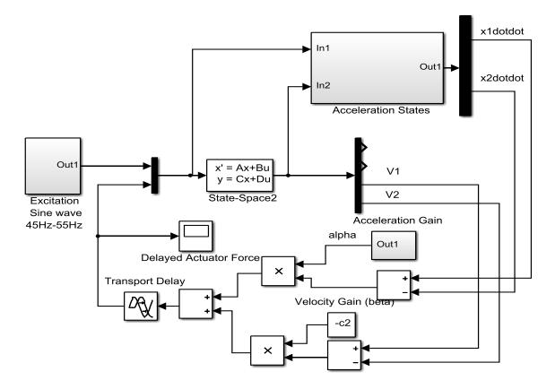
Figure 6-26 SIMULINK model for delayed actuator force with acceleration and velocity feedback
