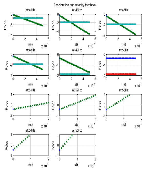
Figure 6-30 System pole variation with acceleration and velocity feedback ignoring the unstable pole before 50Hz
