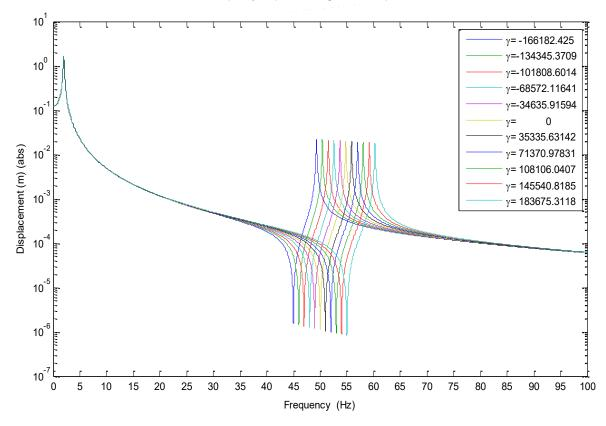
Figure 6-5 Frequency response from excitation force to primary mass displacement with  $\beta = 0$
