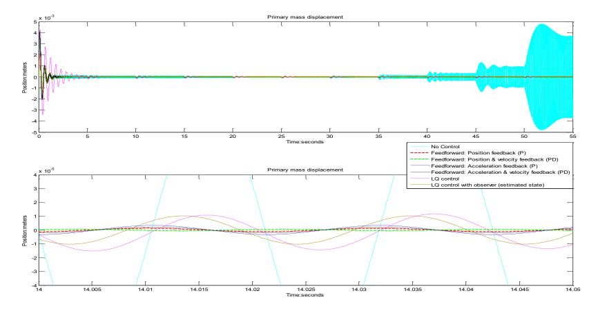
Figure 12-1 Time domain simulation results of the primary mass displacement
