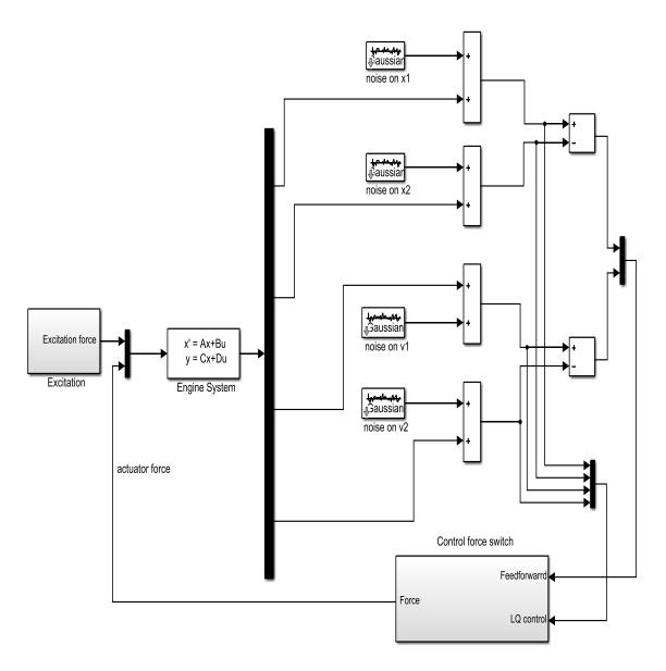
Figure 6-14 SIMULINK with addition of Gaussian noise
