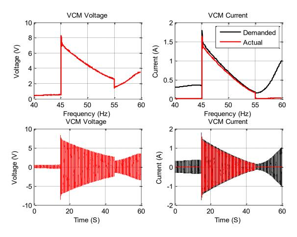
Figure 7-26 VCM voltage and Current with TMD tuned at 55Hz
