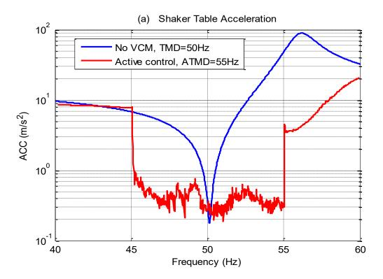
Figure 7-25 Response of the shaker table acceleration with ATMD (originally tuned at 55Hz) vs TMD (originally tuned at 50Hz)
