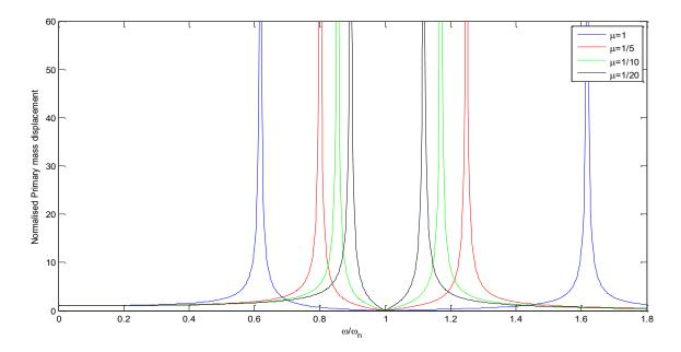
Figure 11-2: Normalised amplitude of vibration of the primary mass as a function of the frequency ratio for several values of mass ratios assuming negligible damping in the primary mass and  $\zeta=0$
