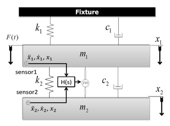
Figure 6-1 ATMD with a 2-DOF system
