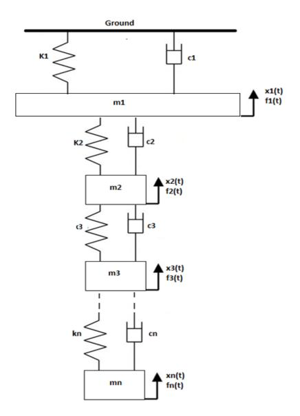
Figure 4-8 Series mechanical tuned mass damper configuration
