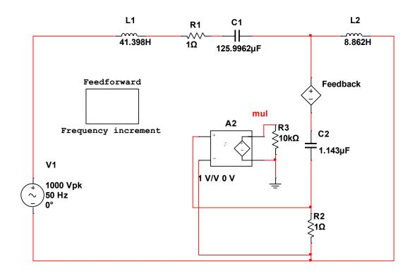
Figure 11-9 Gain scheduling control strategy for the analogous electrical circuit with electrical charge feedback
