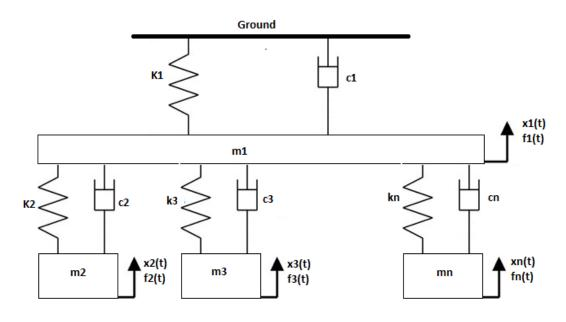
Figure 4-6 Parallel mechanical tuned mass damper configuration
