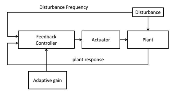
Figure 6-2 Operation principle of the proposed control strategy
