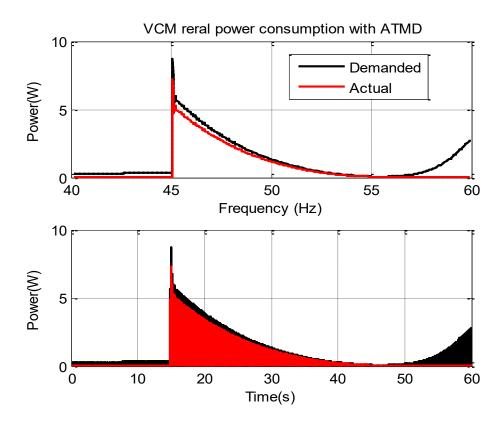
Figure 7-27 VCM Active power consumption with TMD tuned at 55Hz
