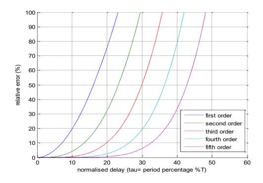
Figure 6-21Percentage error between the original delay function and its Taylor series expansion approximation It is revealed that for the Taylor approximation to be at least 90% accurate, the amount of time delay should not exceed 6% of the value of the operating period T with the first order approximation whereas it can be up to 15% with second order approximation. For the purpose of the application in this research, the first order Taylor approximation is considered.
