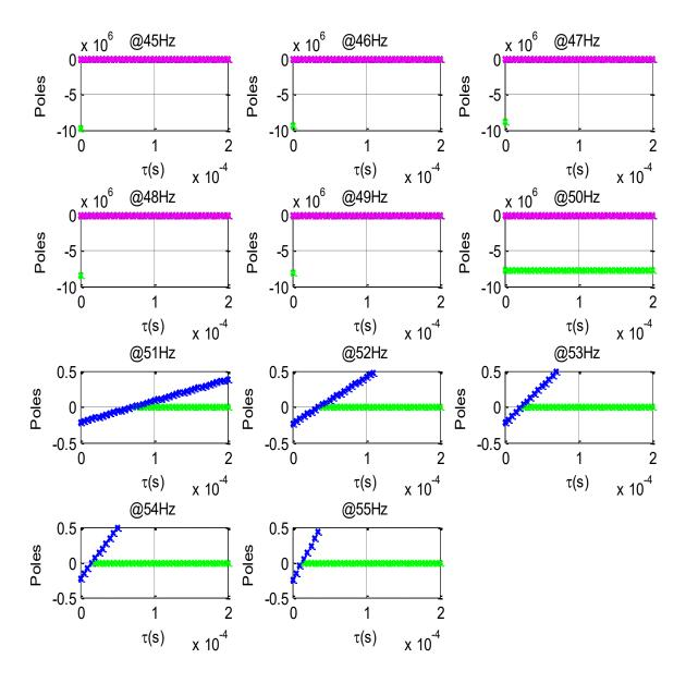
Figure 7-15 Position of the closed-loop poles with gain scheduling control: Acceleration and velocity feedback control with ATMD tuned at 50Hz
