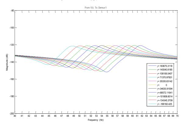
Figure A-6 Frequency response of the primary mass displacement with position and positive velocity feedback
