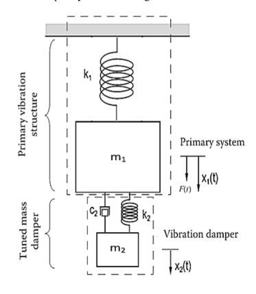
Figure 4-1 2DOF TMD system (Tong, 2014)
