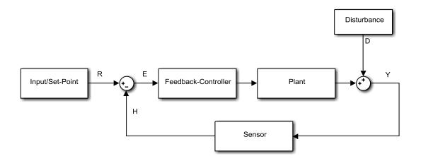
Figure 2-1 Principle of feedback control
