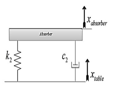
Figure 5-11 Schematic model of the absorber test
