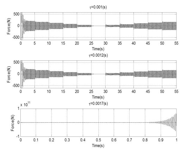
Figure 6-33 Time domain response of the control force with LQ control
