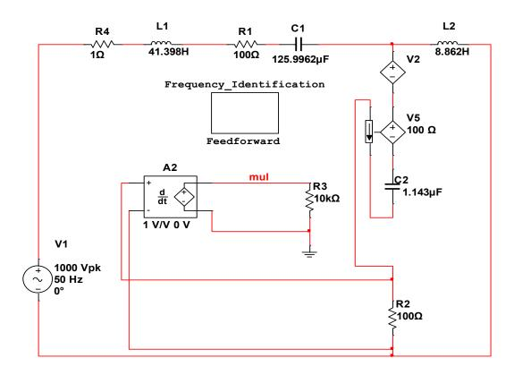
Figure 11-15 Multisim Model with rate of change of electrical charge and electrical current scheduling control strategy
