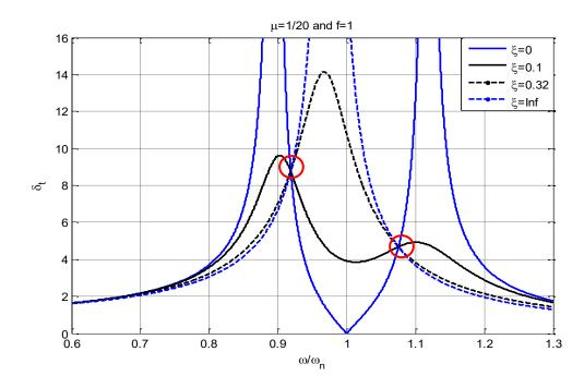
Figure 4-2 Normalised amplitude of vibration of the primary mass expressed as a function of the frequency ratio for different damping ratios and mass ratio  $\mu$ =0.05
