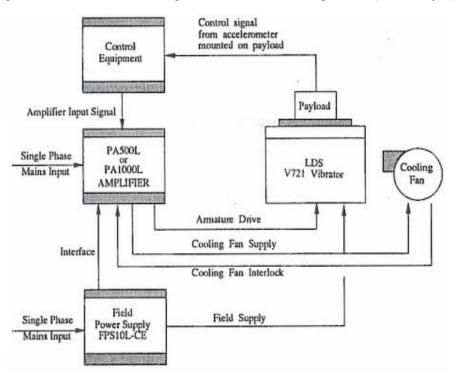
Figure 5-4 V721 series vibrator with PA1000L amplifier and FPS10L field power supply (Bruel & Kjaer)
