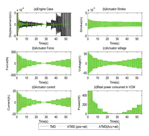
Figure 8-2 Simulation results of the active damping control for the Stirling engine
