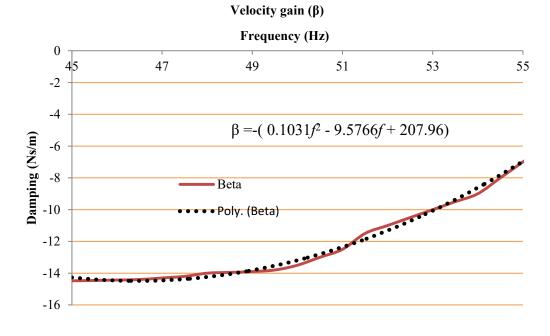
Figure 7-23 Velocity gain against excitation frequency
