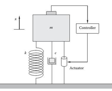
Figure 3-6 General active vibration suppression with feedback control (Tong, 2014)
