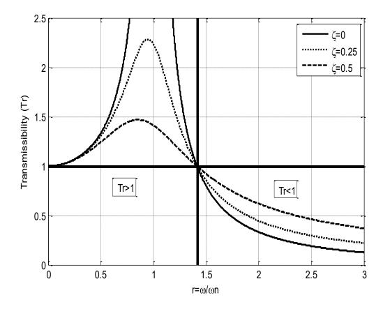
Figure 3-5 The variation of transmissibility with frequency
