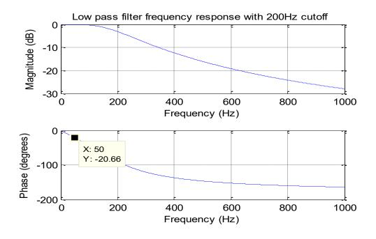
Figure 7-28 Low pass Butterworth filter response with cut-off frequency of 200Hz
