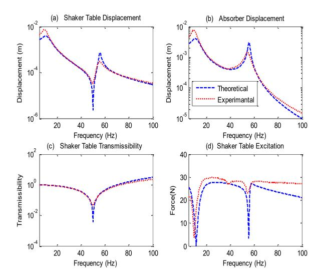
Figure 7-7 Theoretical model results vs experimental results with open circuited VCM
