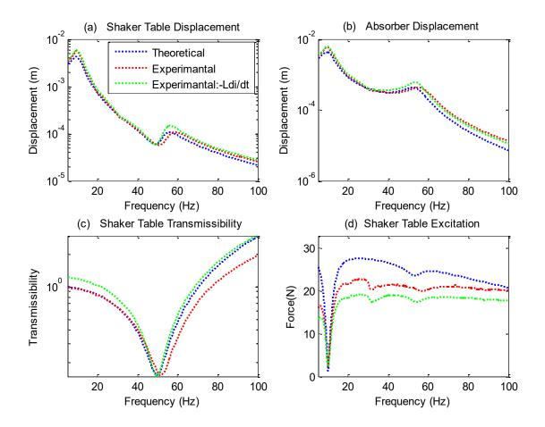
Figure 7-11 Updated theoretical model results vs experimental results with short circuited VCM
