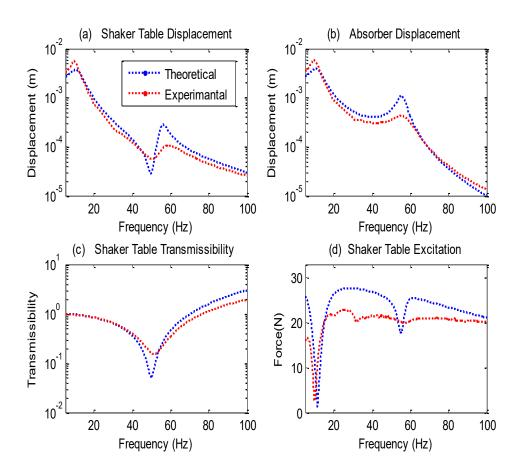
Figure 7-9 Model verification with short circuited VCM
