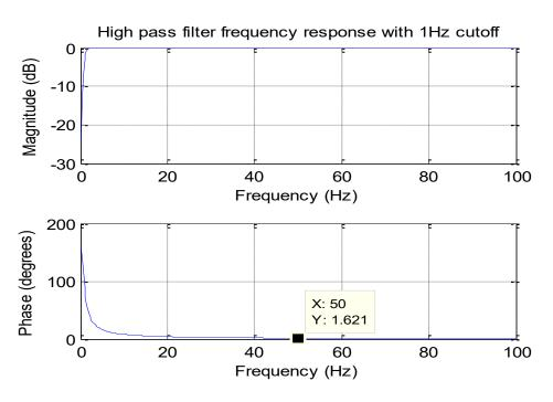
Figure 7-29 High pass Butterworth filter response with cut-off frequency of 1Hz
