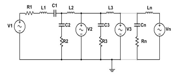
Figure 4-9 Series analogous electrical configuration
