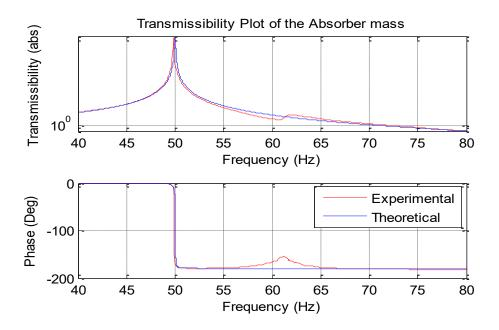
Figure 5-12 Theoretical Vs. Experimental data of the absorber transmissibility. The value of  $c_2 = 2.7 Ns/m$  is determined by reverse fitting of the theoretical data with the experimental data
