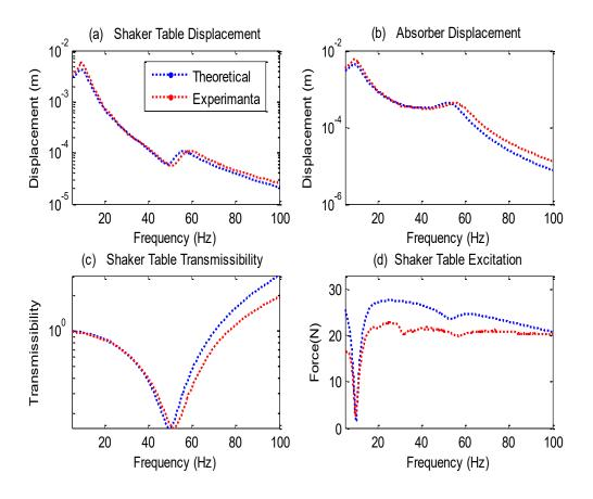
Figure 7-10 Short-circuited VCM with damping  $c_2 = 20.5 Nm/s$
