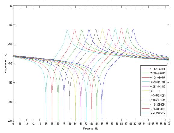
Figure 11-6 Frequency response of the primary mass displacement with position and negative velocity feedback
