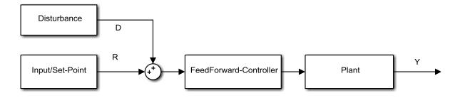
Figure 2-2 Principle of feedforward control
