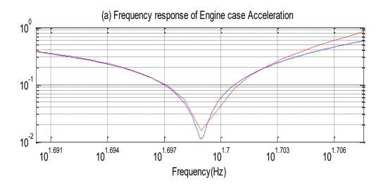
Figure 5-10 Theoretical simulation and experimental validation of the engine
