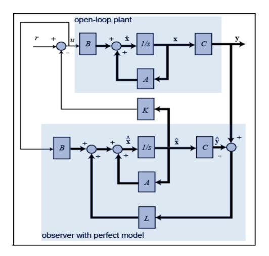
Figure 6-9 Closed loop state observer design (Messner and Tilbury, )
