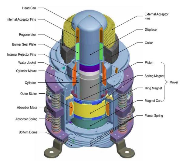
Figure 3-8 Stirling Engine (Microgen Engine Corporation, )
