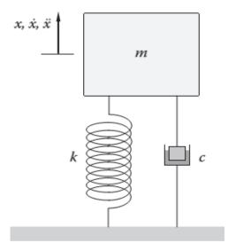
Figure 3-2 Spring-mass system with viscous damper (Tong, 2014)
