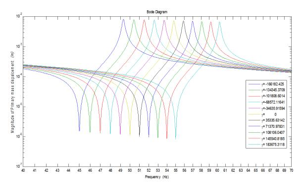
Figure 11-4 Frequency response of the primary mass displacement with position feedback
