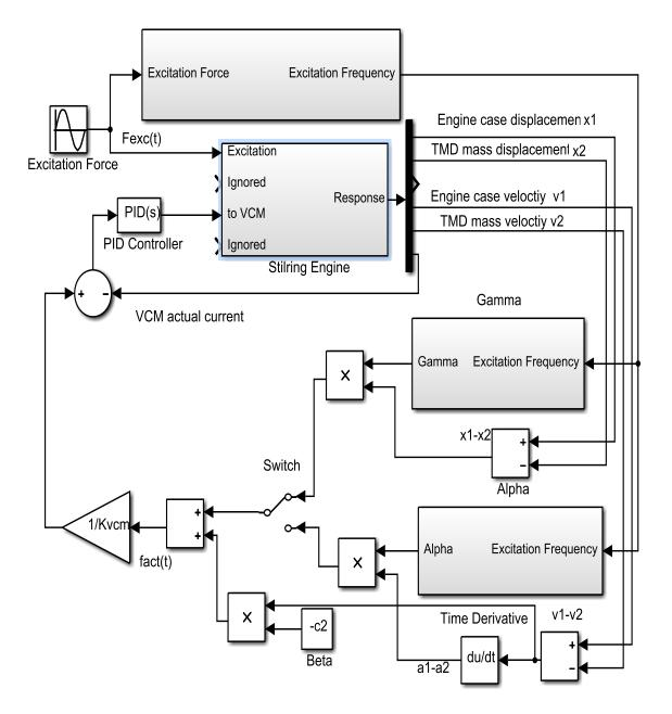
Figure 8-1 Schematic model diagram for the active damping control of the Stirling engine
