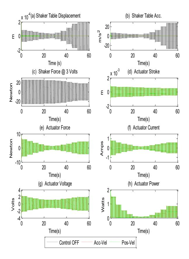
Figure 7-13 Time domain simulation results for the active damping control of the designed rig
