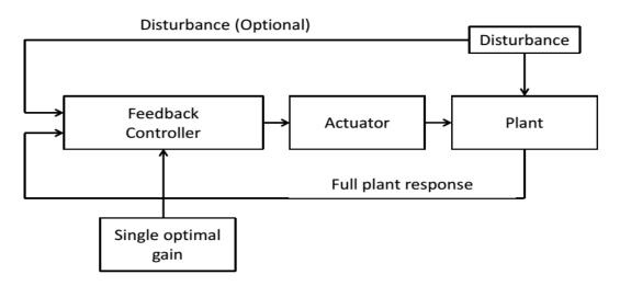
Figure 6-7 Operation principle of the LQ control
