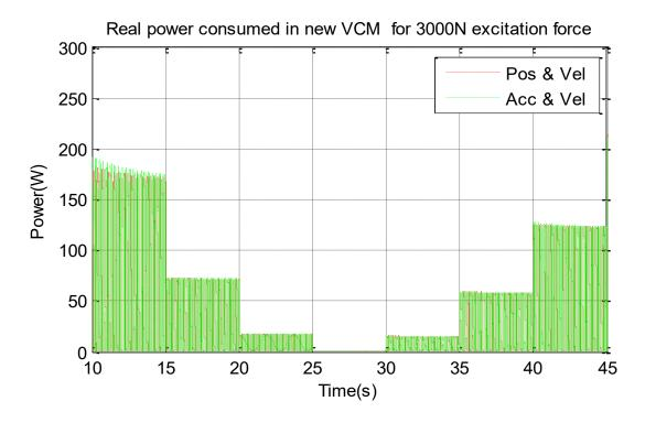
Figure 8-4 Real power consumption of the VCM for 3kN excitation force and VCM motor constant  $k_{vcm} = 51.6 [N/A]$
