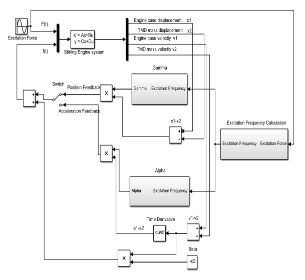
Figure 11-3 SIMULINK model used to simulate the control of the engine vibration with ATMD
