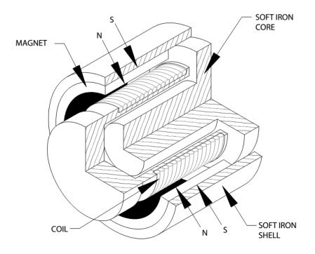
Figure 3-10 Conventional construction of a VCM (Kimco Magnetics)
