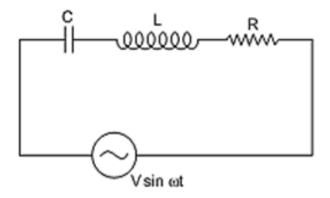
Figure 4-5 Driven LRC circuit
