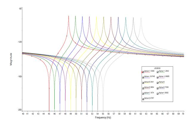
Figure 11-17 Frequency response with current and negative rate of change of current feedback
