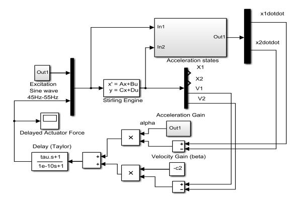
Figure 6-28 SIMULINK model with delay represented as per Taylor approximation
