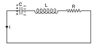
Figure 4-4 LRC circuit
