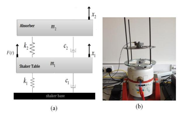
Figure 7-1 Initial test rig
