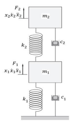
Figure 3-3 Two degrees of freedom spring-mass system with viscous damping (Tong, 2014)
