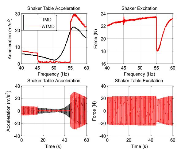
Figure 7-31 Shaker table excitation and acceleration with TMD tuned at 50Hz with delay cancelation
