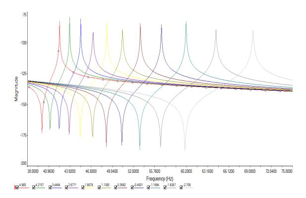
Figure 11-11 Frequency Response with current rate of change feedback gains
