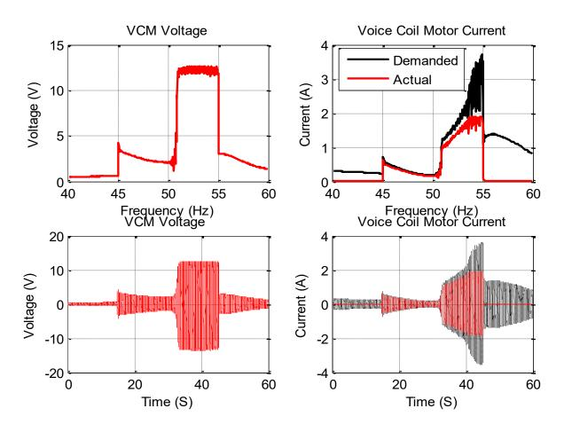
Figure 7-21 Test1: VCM voltage and Current with active control
