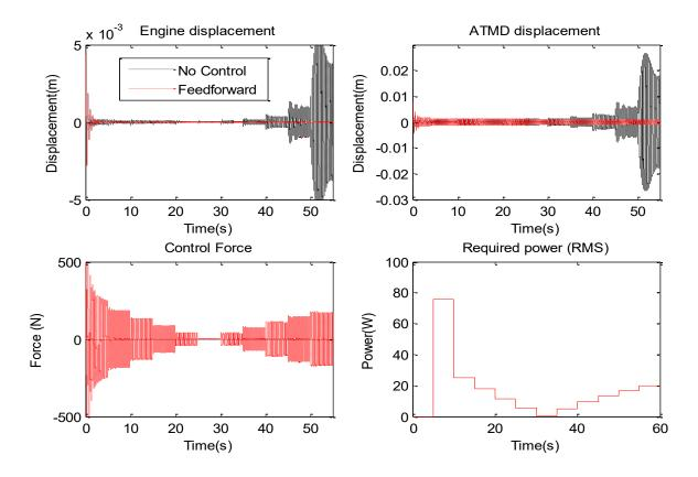
Figure 6-12 Simulation results with gain scheduling control (position feedback)
