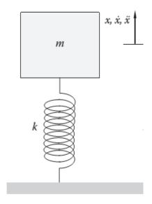
Figure 3-1 SDOF Spring-mass system free body diagram (Tong, 2014)
