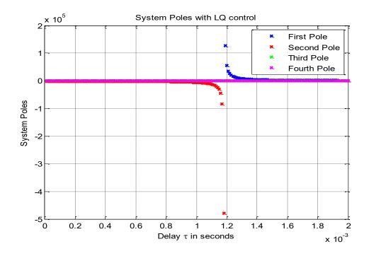
Figure 6-32 System poles variation with LQ control
