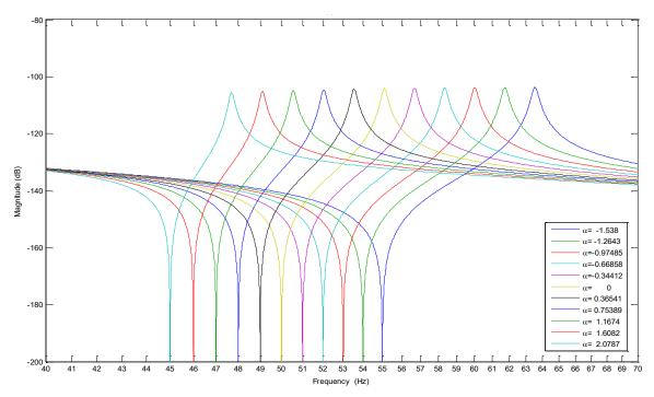
Figure 11-8 Frequency response of the primary mass displacement with acceleration and negative velocity feedback
