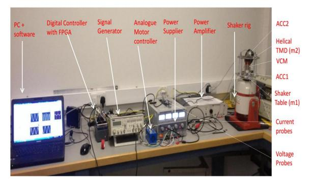
Figure 7-18 Active damping shaker-absorber rig
