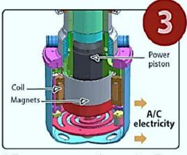
3. The pressure wave moves the power piston. The power piston includes magnets which move past a stationary coil producing alternating electrical current.
