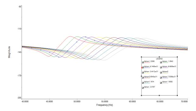
Figure 11-16 Frequency response with rate of current and with positive rate of change of current feedback gain
