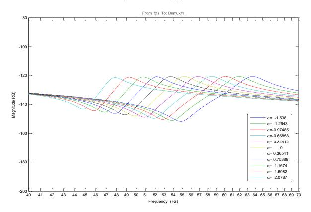
Figure 11-7 Frequency response of the primary mass displacement with position and with positive velocity feedback
