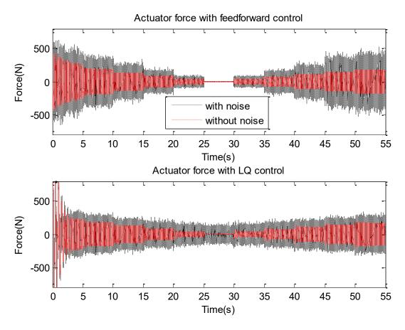
Figure 6-16 Effect of noise on the actuator force with each control strategy
