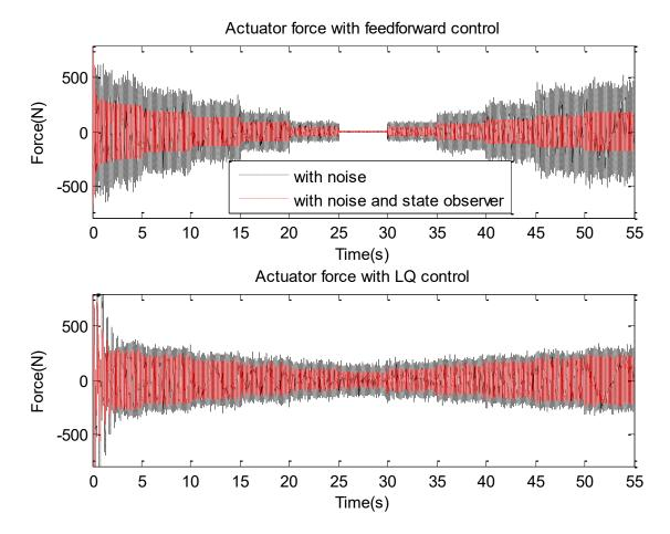
Figure 6-18 Noise mitigation with of state observer on noisy signals
