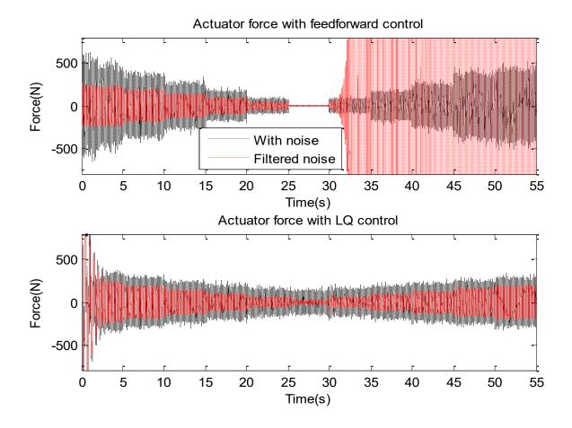
Figure 6-20 Noise mitigation with of low pass filtering of noisy signals
