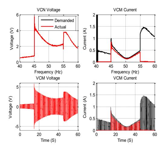
Figure 7-32 VCM voltage and Current with TMD tuned at 50Hz with delay cancellation
