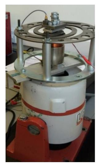
Figure 7-6 Shaker with absorber and VCM test rig
