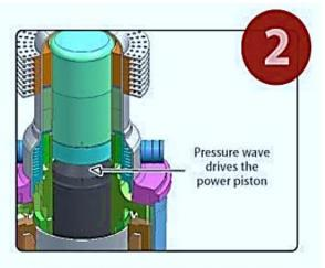
2. As the Helium is alternately heated and cooled, it expands and contracts, creating a pressure wave inside the generator.
