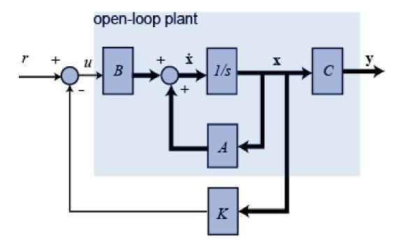
Figure 6-8 Schematic representation of LQ control state space system (Messner and Tilbury, )
