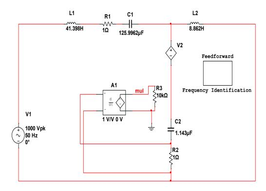
Figure A-12 Gain Scheduling control strategy for the analogous electrical circuit with acceleration feedback
