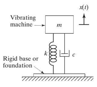
Figure 3-4 SDOF representation of an isolation system with rigid foundation (Rao, 1990)
