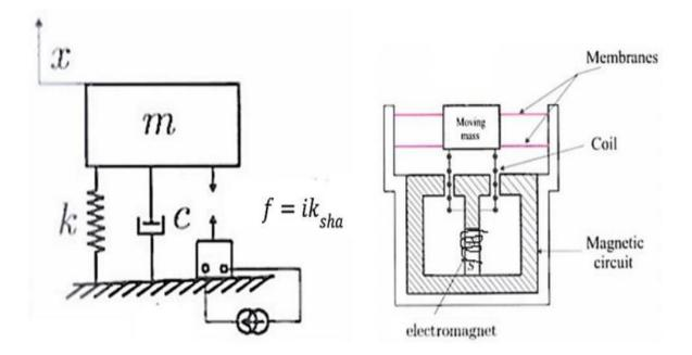
Figure 5-5 Schematic of the design of an electrodynamic actuator (Preumont, 2012)
