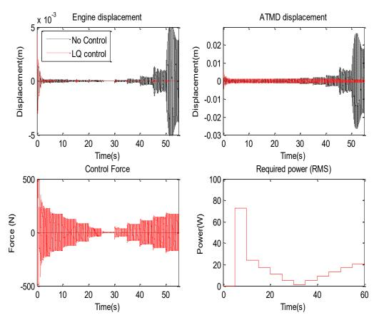
Figure 6-13 Simulation results with LQG control (based on estimated states)
