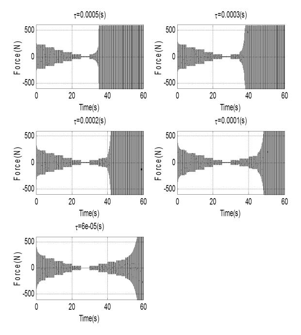
Figure 6-31Time domain response of the control force with acceleration and velocity feedback
