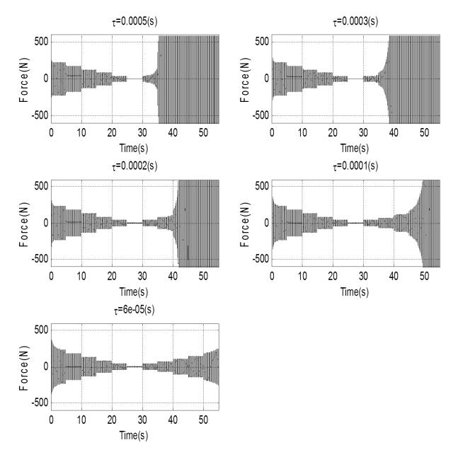
Figure 6-24 Time domain response of the control force with acceleration and velocity feedback with positive time delay showing system instability after 50Hz for different time delays
