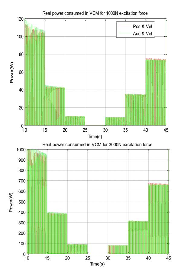
Figure 8-3 Close-op view of the real power consumption of the VCM for 1kN and 3kN excitation forces
