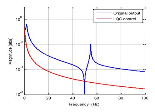
Figure 6-11 Engine case displacement with original system Vs. LQG control
