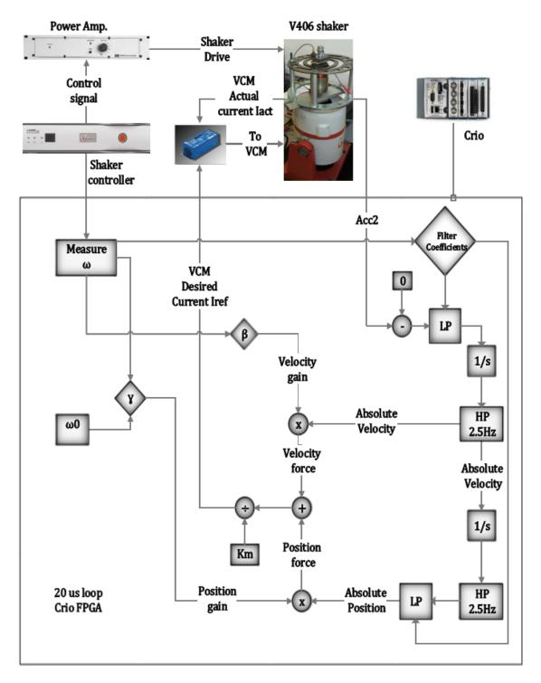
Figure 7-34 Schematic Diagram of the control model of Test 4
