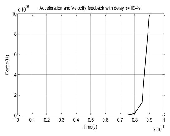
Figure 6-29 Time domain response with Taylor representation of time delay
