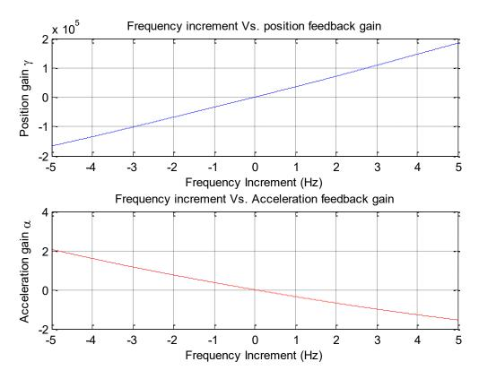
Figure 6-3 Required values of gains  $\gamma$  and  $\alpha$  to produce a frequency shift of 10 Hz bandwidth
