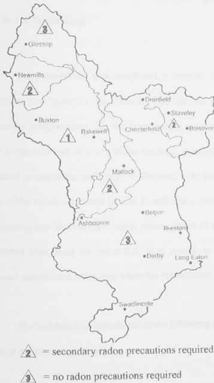
Figure 5.3.1. Radon Map of Derbyshire With Radon Precautions Requirement for New Dwellings (BRE, 1992)
