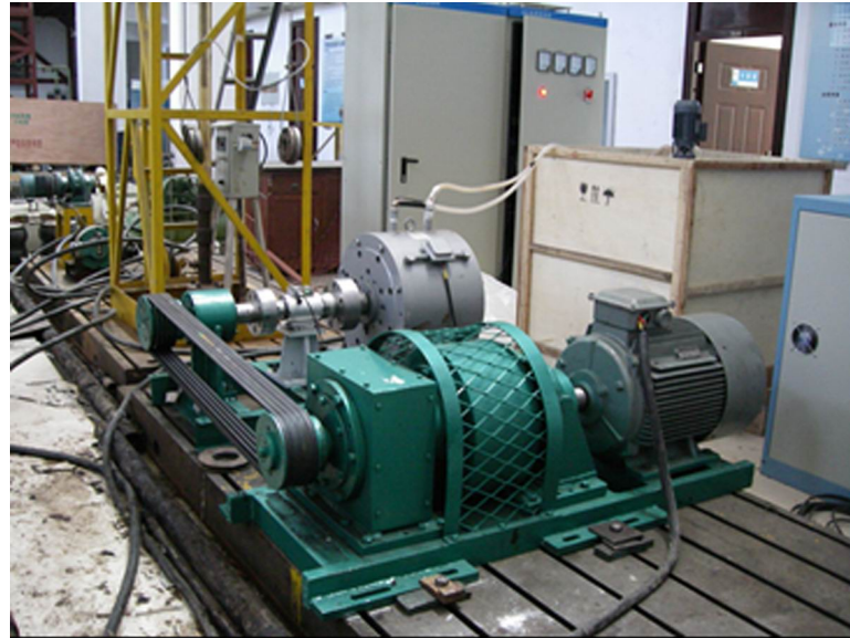
Fig 1. Experimental apparatus for external characteristics of the motor.
