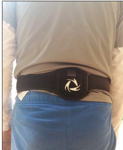
Figure 5.5 The G-Walk attached to the participant’s waist using a semi-elastic belt covering the L4-L5 intervertebral space.
