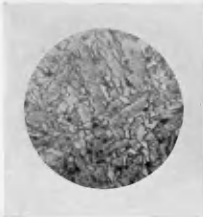
FIG. 68—Nickel steel 6. Heated for 12 hours at 685° C. and water-quenched. Etched with alcoholic 1 per cent. nitric acid and boiling alkaline sodium picrate. \times 600 .
