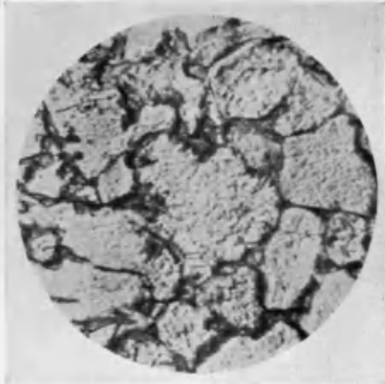
FIG. 69—Nickel steel 2. Heated for 12 hours at 700° C. and water-quenched. Etched with alcoholic 1 per cent. nitric acid. \times 600 .
