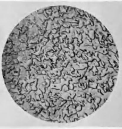
FIG. 78—Nickel steel 6. Heated for 24 hours at 705° C. and water-quenched. Etched with alcoholic 1 per cent. nitric acid. \times 600 .
