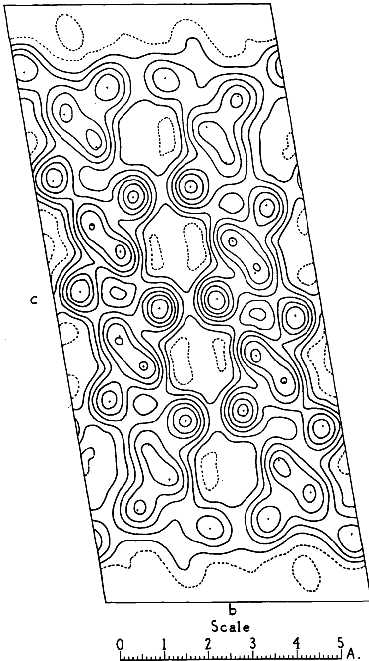
Fig. 20. Projection of the tetracene structure along the a crystal axis, drawn on the (100) plane. Each contour line represents a density increment of one electron per \text{\AA}^2 , the one electron line being dotted.
