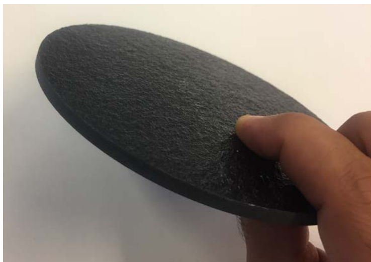
Figure 2: 100 mm diameter sample after autoclave and cut by water jet cutting.
