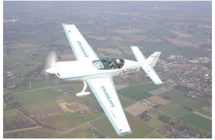
Fig. 9. The Extra 330LE aerobatic plane, powered by a lightweight hybrid-electric propulsion system, set a new record when it reached 337.5 km/h [40].
