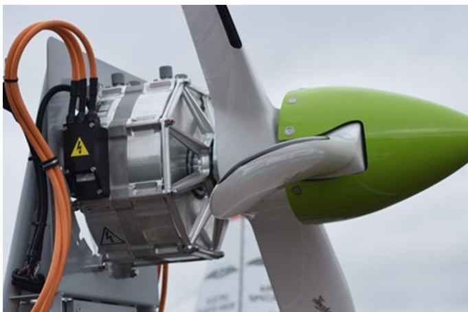
Fig. 2. High-density YASA electric motor for the Electroflight P1e [11].
