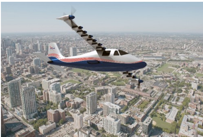
Fig. 5. NASA's X-57 distributed thrust Electric Research Plane [21].
