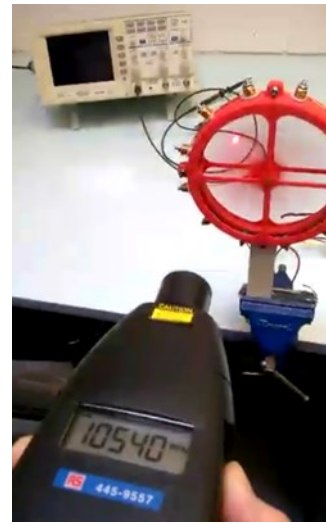
Fig. 6. Prototype RDF unit running at speeds in excess of 10,000 rpm.
