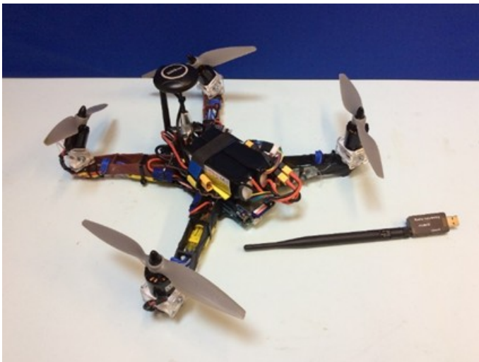
Fig. 2. V-tail Quadcopter configured with a data-logger and telemetry for validation flight testing.
