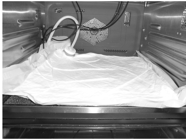
Fig. 8. Bagged composite prior to curing. Three FOTs enter the left side of the bag from the top of the oven; the vacuum port is situated at the back right-hand side. The composite is covered with release film, wrapped in breather and bagged. “Tacky tape” seals the bag and vacuum line. The vacuum puck is microwave-transparent PTFE.
