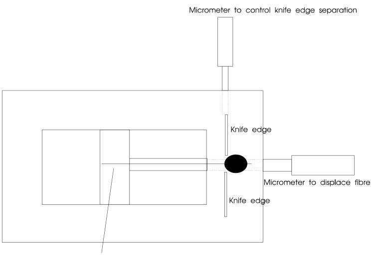
Fibre adhered to moving block
